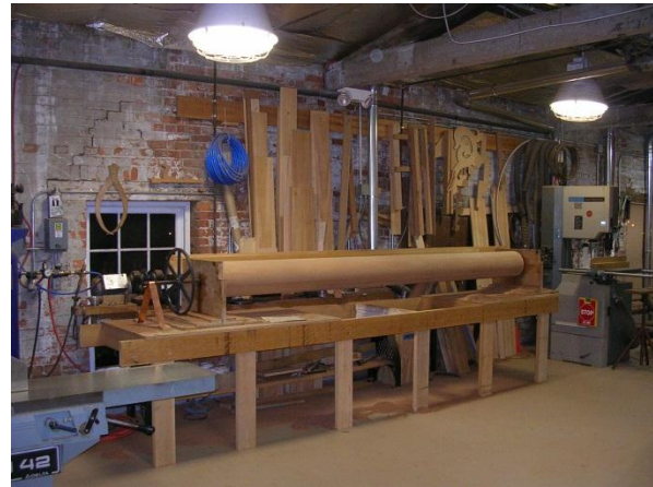
Figure 8 : Mahogany lumber was milled, cut on a bevel, glued with tight bond III glue, and clamped together. The rough laminated columns were then turned on the lathe and machined to a smooth round column.
