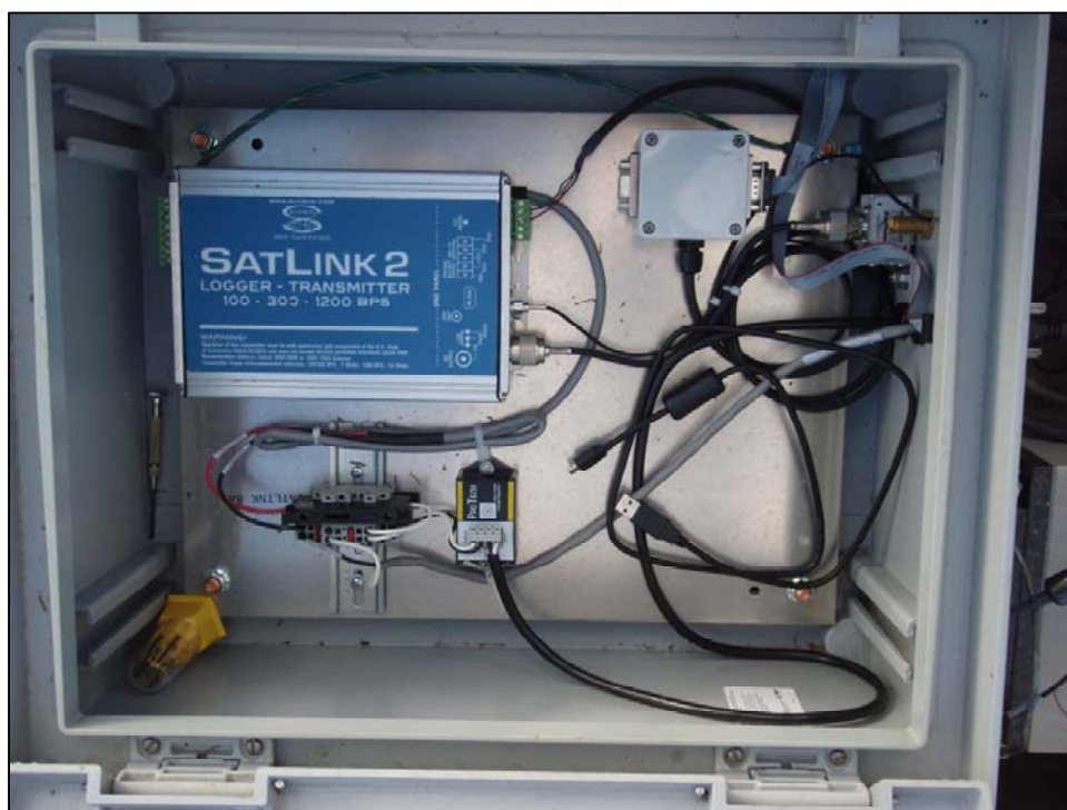
Figure 3. Data Collection Platform system at the Delaware River at Lordville, NY continuous water-quality monitoring site that is maintained by the Eastern Rivers and Mountains Network.
