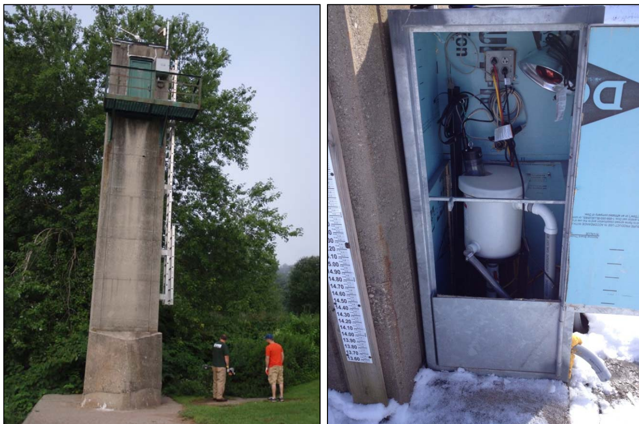
Figure 4. Continuous water-quality monitoring system, maintained by the Eastern Rivers and Mountains Network, that is located at the Delaware River near Montague, NJ. The data collection platform and telemetry equipment are located near the top of the U.S. Geological Survey concrete tower (left) whereas the flow through basin and monitor are located in a galvanneal steel shelter adjacent to the tower.
