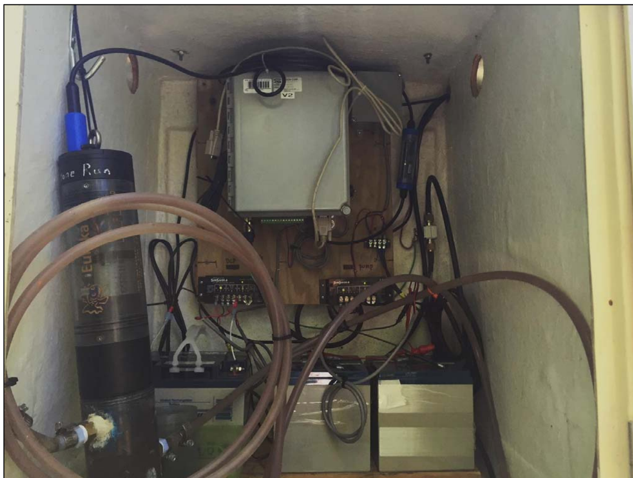
Figure 2. Continuous water-quality monitoring system located at the Delaware River near Delaware Water Gap, PA.
