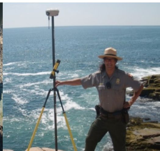
Figure 3. Above left: an example of an embedded NPS survey monument. These monuments serve as stable reference points when collecting elevation data. Above right: A park ranger uses a survey monument (beneath the center tripod leg) to position an RTK-GPS instrument. Photos by Michael Bradley, URI EDC.
