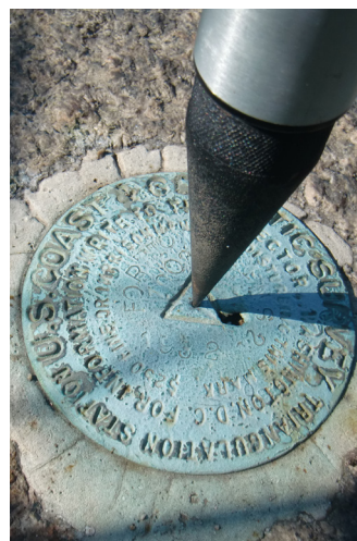
Figure 3. Above left: an example of an embedded NPS survey monument. These monuments serve as stable reference points when collecting elevation data. Above right: A park ranger uses a survey monument (beneath the center tripod leg) to position an RTK-GPS instrument. Photos by Michael Bradley, URI EDC.
