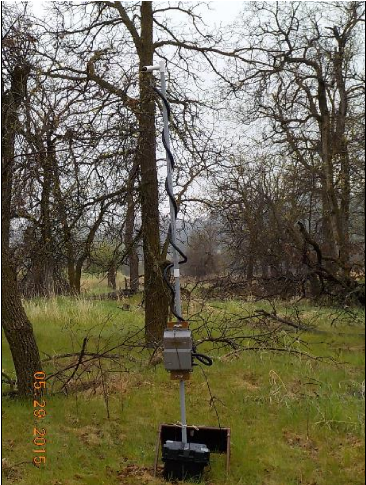
Figure 3. Example of the acoustic monitoring equipment deployed at DETO.
