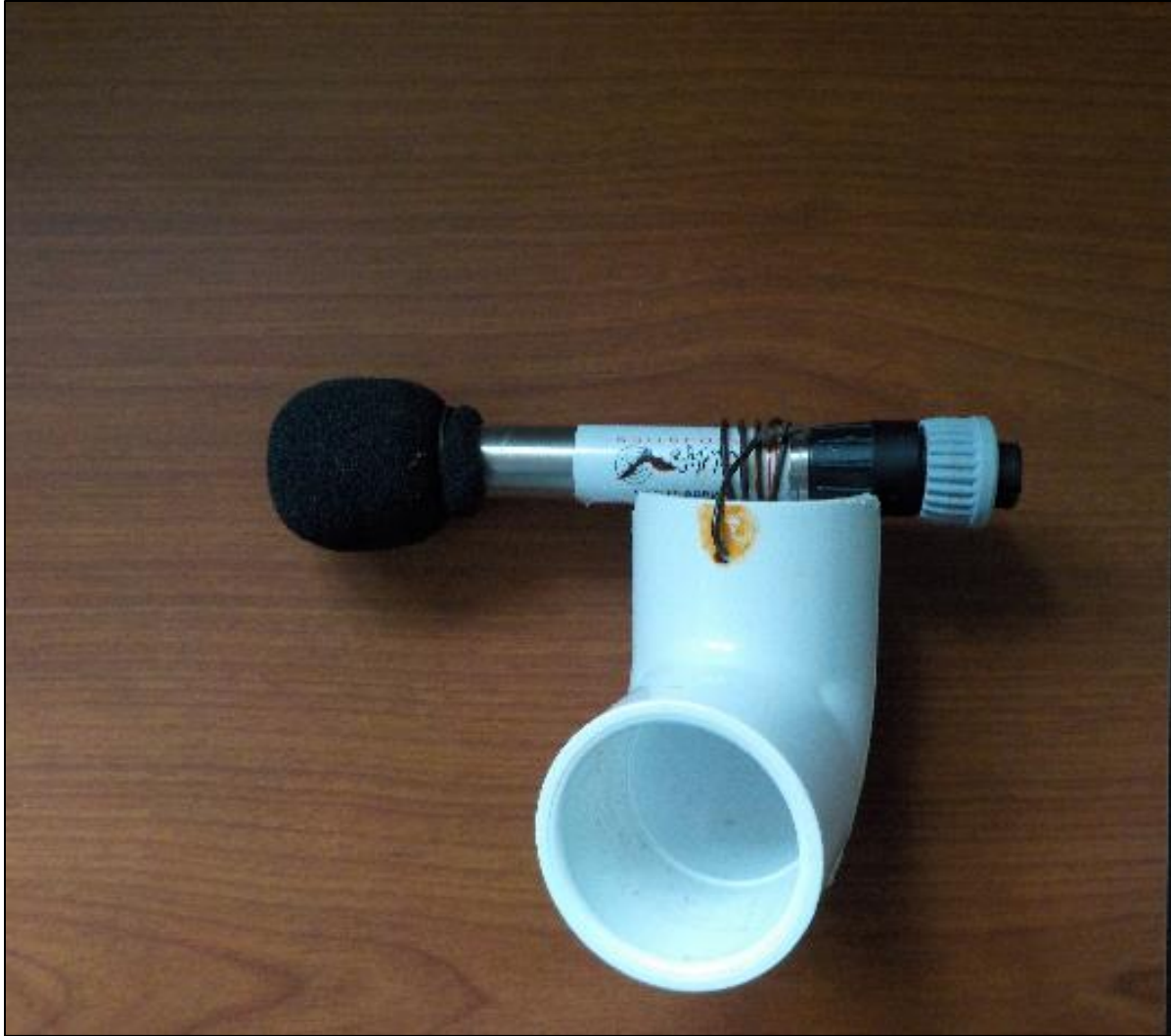
Figure 2. Photograph illustrating microphone attachment. Note that this microphone is a newer model than what was used for this study. Prior models had holes at the base that could be screwed into the connector piece.
