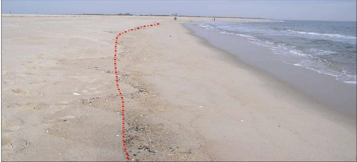
Figure 7. The high-tide swash line (red dashed line) has small irregularities that will be smoothened, recording the average position of the line (Figure from Psuty et al. 2010).
