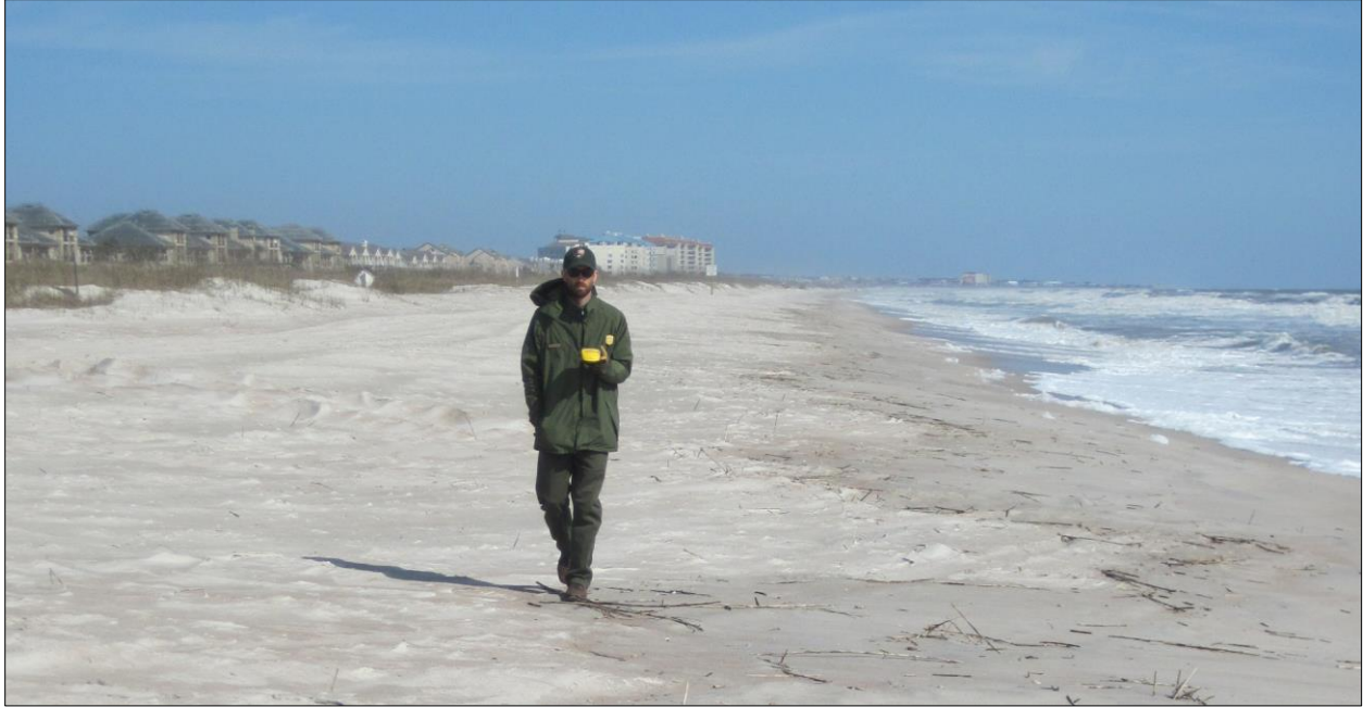
Figure 8. Conducting the survey and holding the GPS receiver. The operator walks along the wet/dry line on the beach face to capture the position of the neap high-tide swash line.
