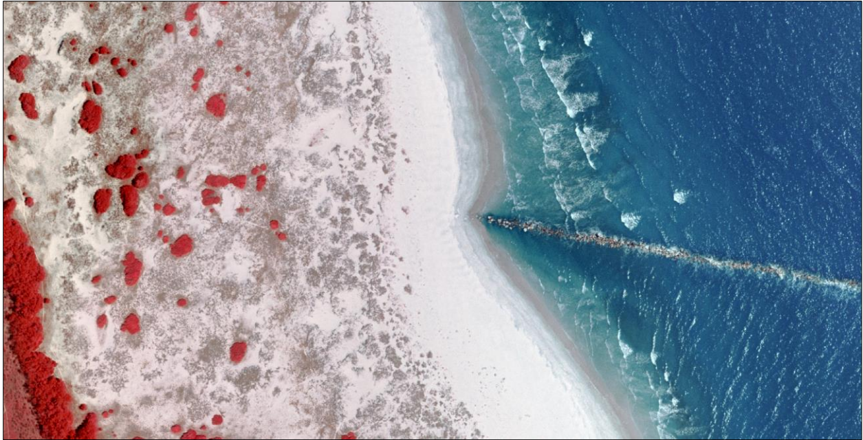
Figure 9. This aerial view of GATE-SHU demonstrates how an interruption source offsets the shoreline. Source: NPS-GATE (Figure from Psuty et al. 2010).
