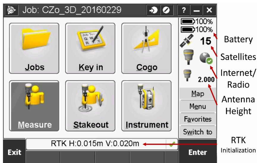
Figure S5.1. Example of a Trimble R10 Survey Controller screen showing information about the rover unit status.
