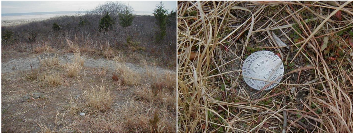
Figure S2.2. The monument PID KU2138 located in the field at Gunnison Beach, Sandy Hook Unit, Gateway National Recreation Area. Note the designation that is inscribed on the disk and assigned to it as an identifier by the NGS, “FALSE”, that is also noted on the datasheet associated with this monument in Figure S2.3.
