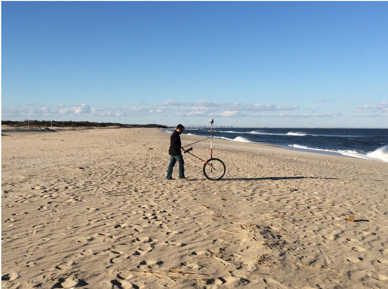
Figure S5.4. Survey wheel constructed to facilitate the collection of topographical data.
