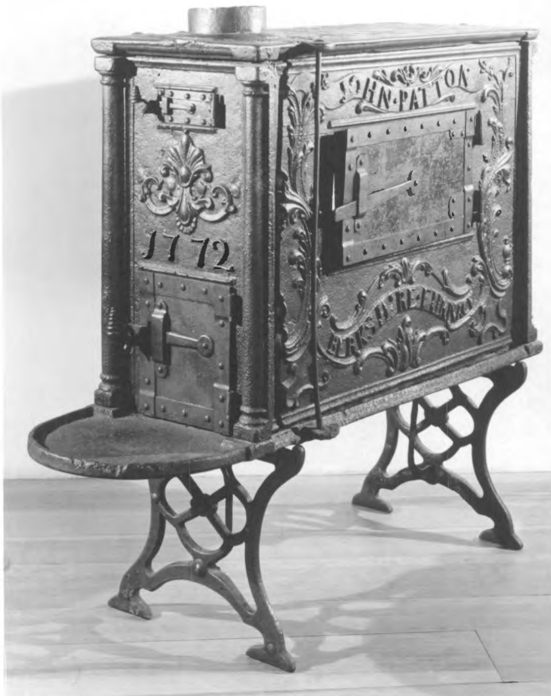
Illustration #29. Pennsylvania cast iron ten-plate stove signed: "John Patton, Berkshire Furnace, 1772." The two stoves of local manufacture which were set up in the Assembly Room during the winter of 1771-72 must have closely resembled this one. The rococo decoration of this stove can also be seen in fine Philadelphia cabinet-work of this period. INHP Collection. INHP Neg. #9238.
