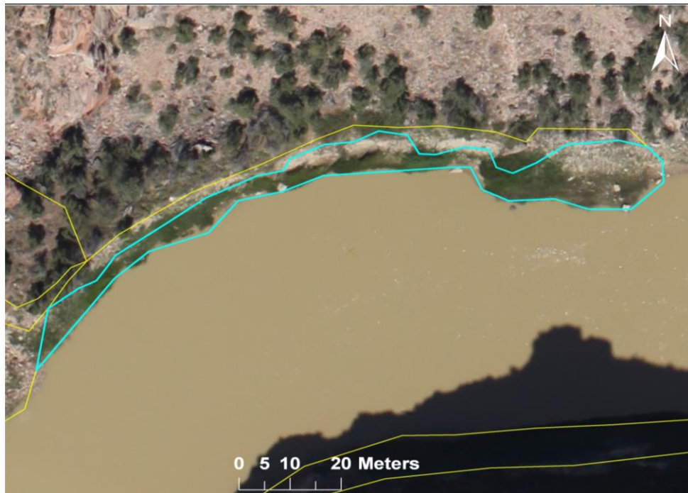
Figure 5. An active channel feature outlined in blue, associated with a pool immediately upstream of a debris fan. In such settings, where shear stresses presumably remain low even during high flows, a guild of active channel plant species (Table 1) can show high cover even within the active channel zone. Such situations are not indicative of channel narrowing unless they are vertically accreting and/or have a persistence presence of flood plain indicator species.
