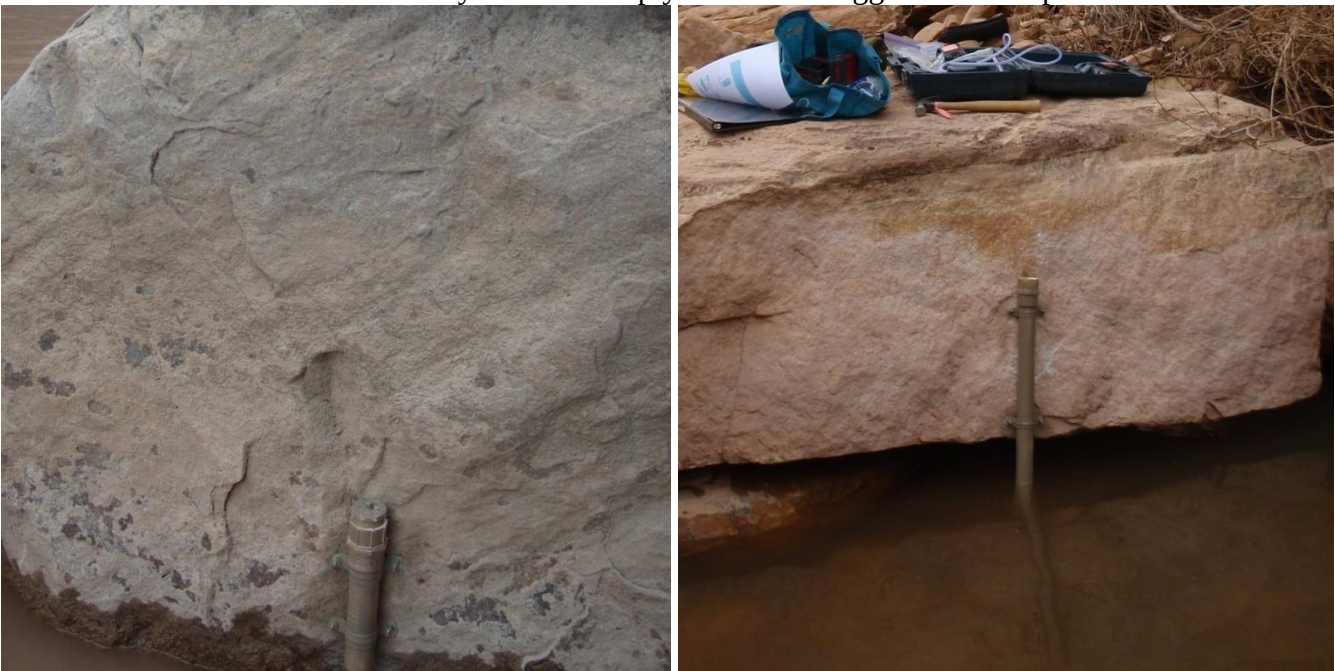
Figure 5. Water transducers attached to boulders and painted to match surroundings.
