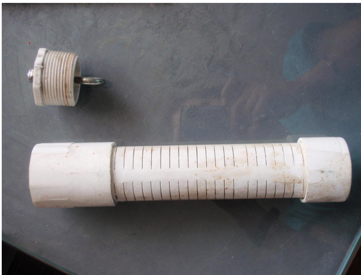
Figure 1. Example of an air transducer casing. A water transducer casing would not have a cap on the bottom.
