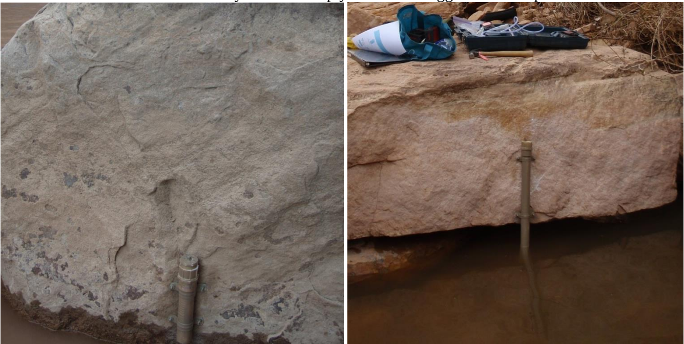
Figure 6. Water transducers attached to boulders and painted to match surroundings.
