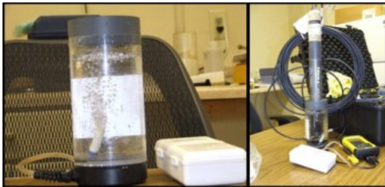
Figure SOP 5-2. InSitu dissolved oxygen calibration chamber with aquarium pump and oxygen stone.
