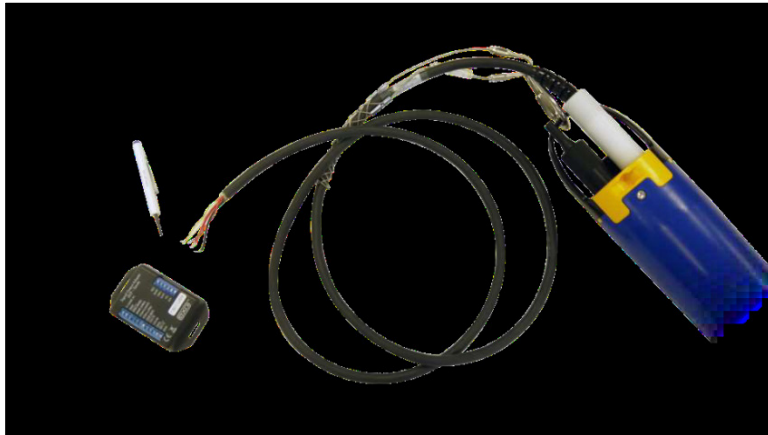
Figure SOP 6-6. YSI 6096 flying lead adaptor (connected directly to datasonde).
