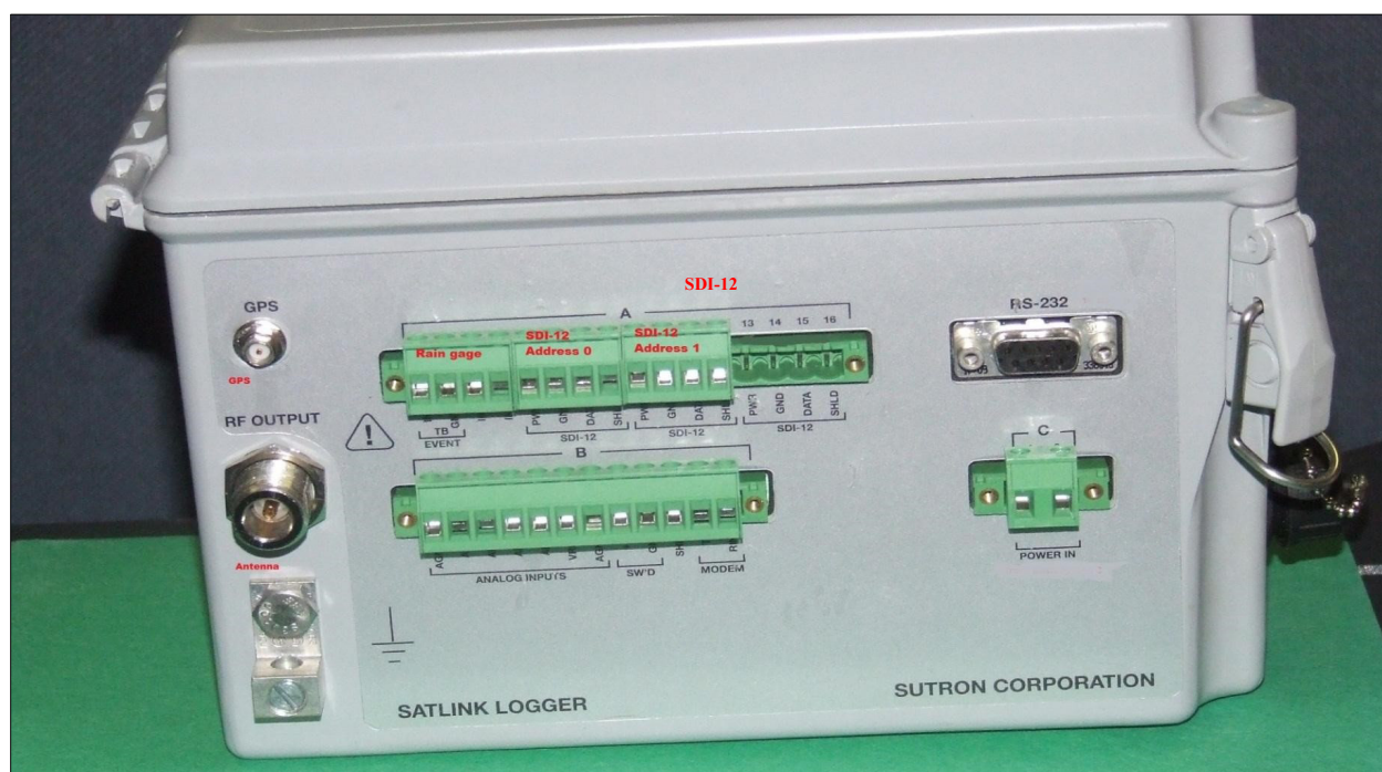
Figure SOP 6-7. Sutron datalogger showing connection boards on rear panel (red annotation added).
