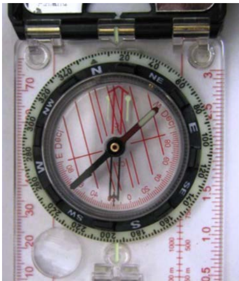
Figure 2.1. Compass displaying components used to find a bearing
