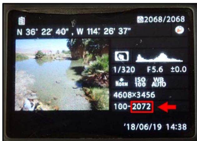
Figure 11.1. Location of the last four digits of the image code (indicated by red arrow) on the review screen of the Olympus TG-4 camera.
