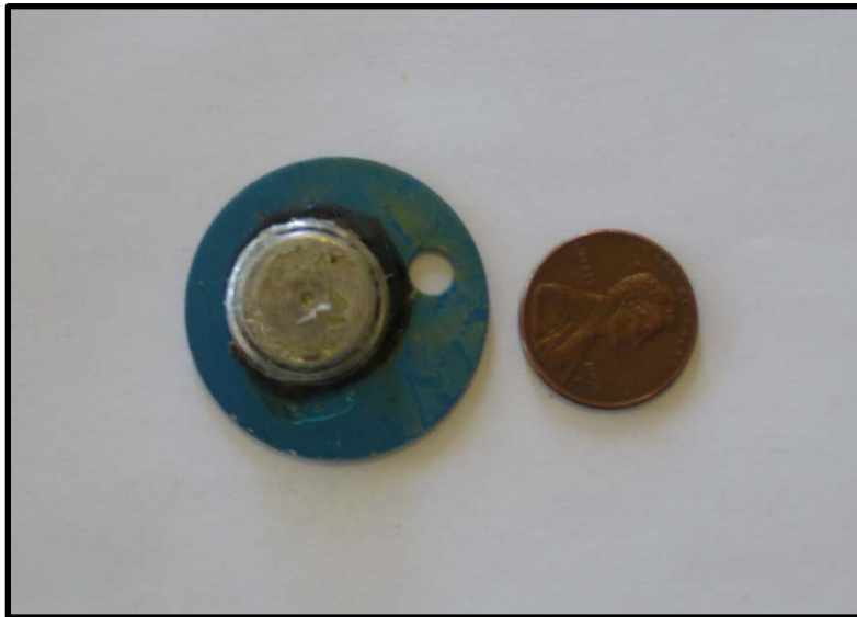
Figure 6.1. iButton epoxied to a metal disk. Penny for scale.
