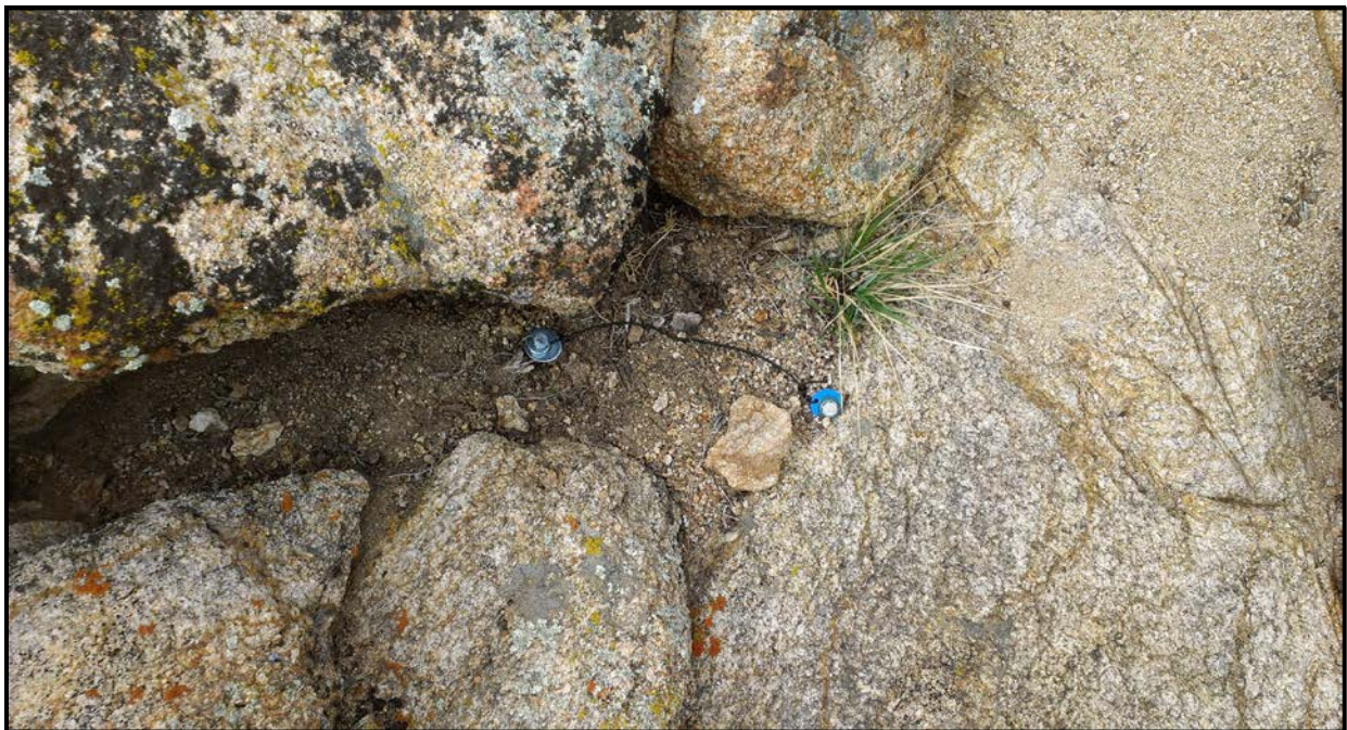
Figure 6.4. Bolt pounded into substrate with tag and sensor attached by electrical wire.
