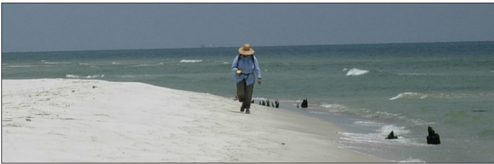
Crew member walking the high tide swash line with a handheld GPS to collect data for the shoreline position protocol.
