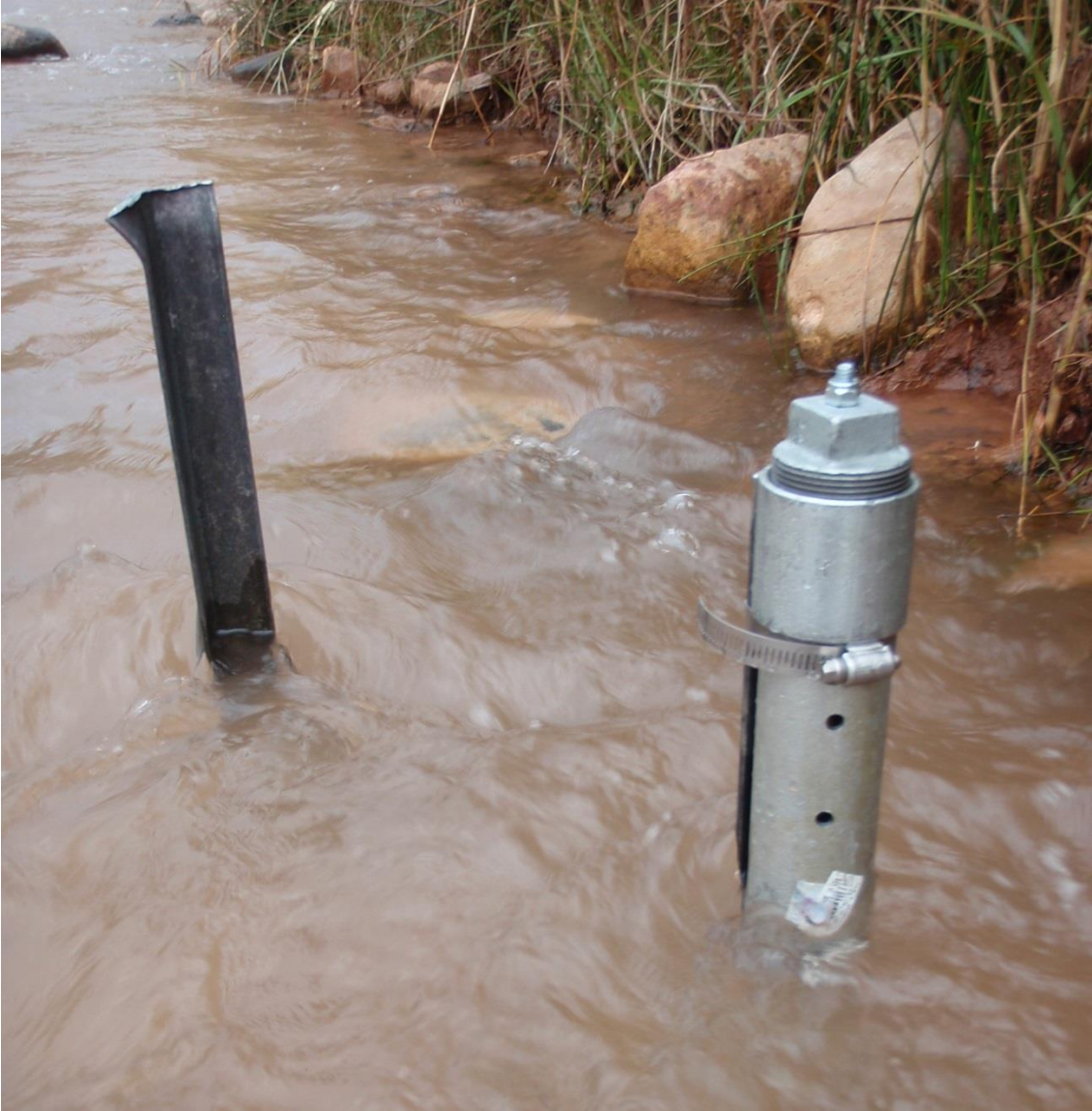
Figure 10. Angle iron installation in the Fremont River, Capitol Reef National Park.
