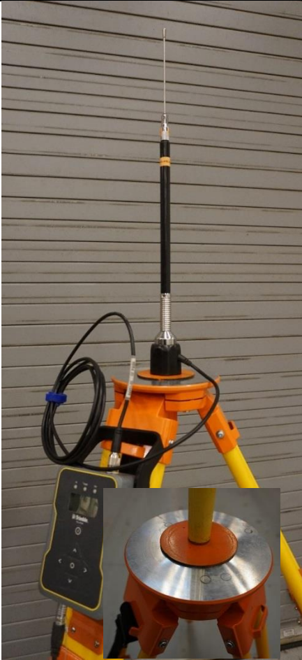
Figure 17 – Base station radio setup
