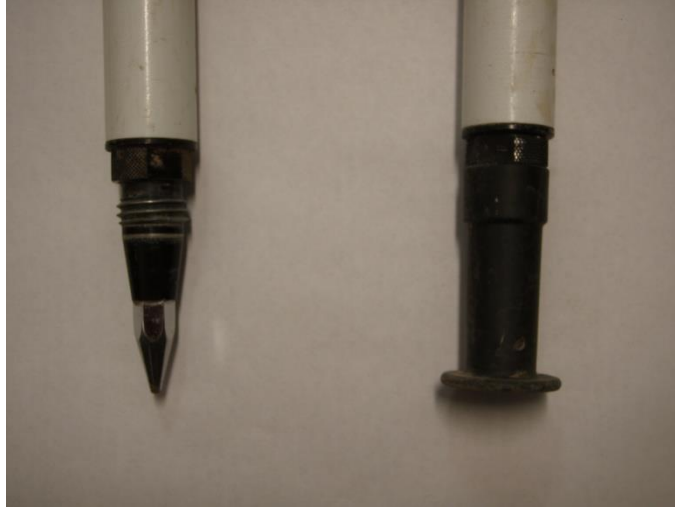
Figure 2. Options for the bottom of prism poles. The point on the left is used for control points, top of headpins, and well shots while the flat foot is on the right is used for all other shots. Leveling rods only have a flat foot.
