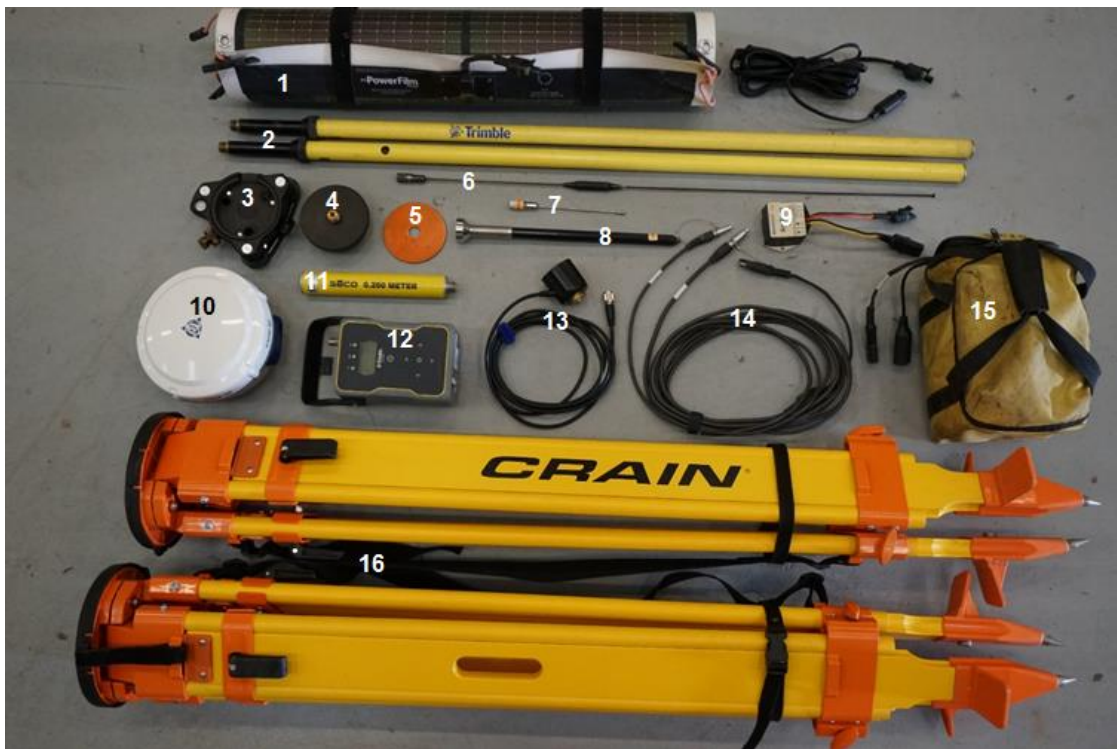
Figure 12 – RTK base station equipment unpacked
