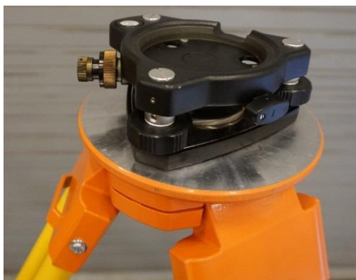
Figure 14 – Base tripod with tribrach base mounted
