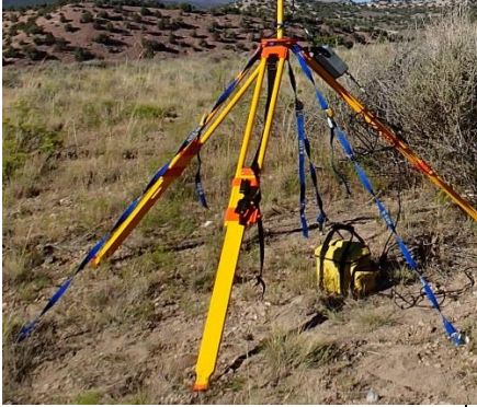
Figure 15 – Base tripod anchored with tie-down straps
