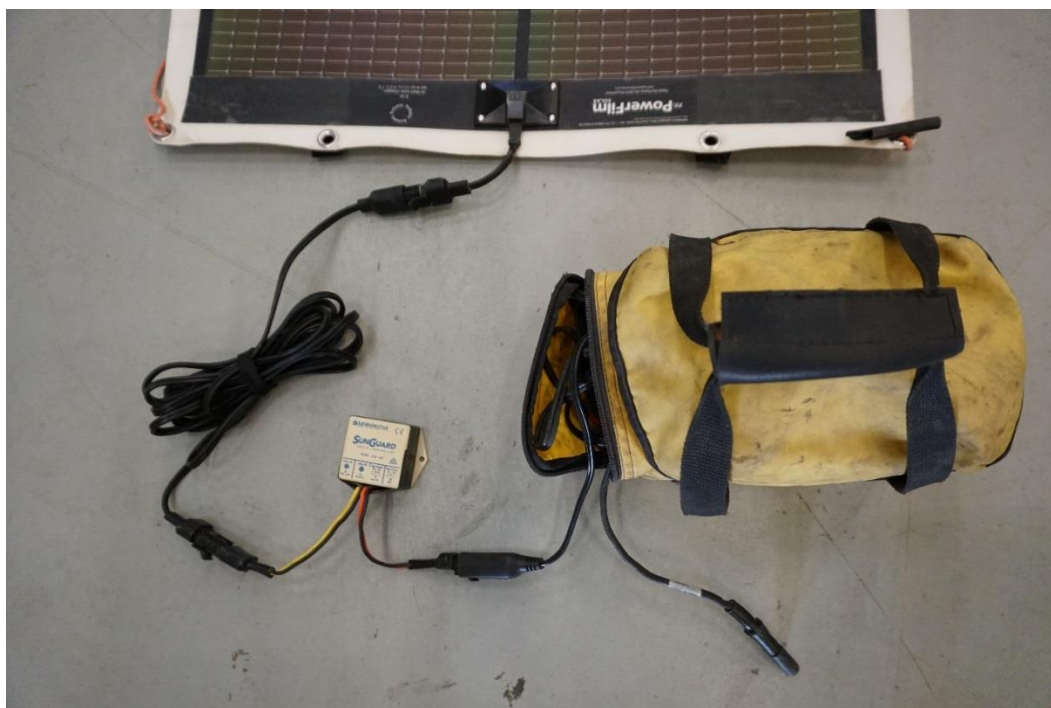
Figure 18 – Base station battery and 42 watt solar panel charging system
