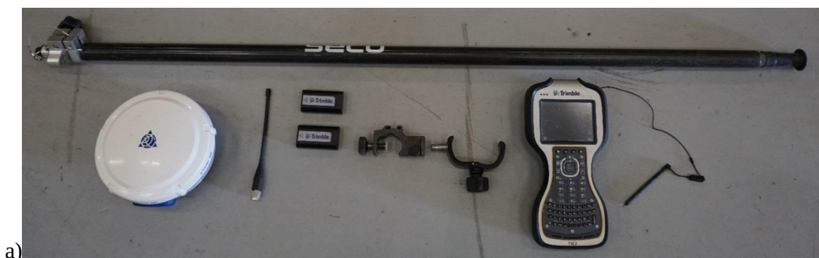
Figure 20 – Trimble R6 rover a) pelican case containing rover survey gear and accessories b) rover survey gear unpacked
