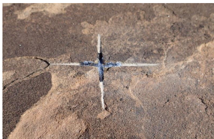
Figure 9 – Example of base station cross/plus etched into rock surface
