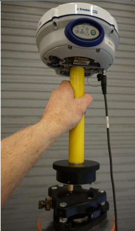
Figure 16 – Base station receiver setup
