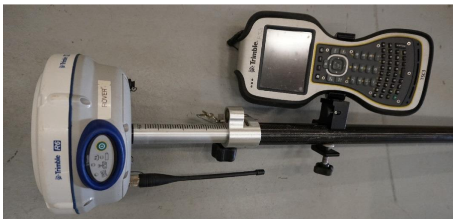
Figure 21 – Trimble R6 rover gear assembled
