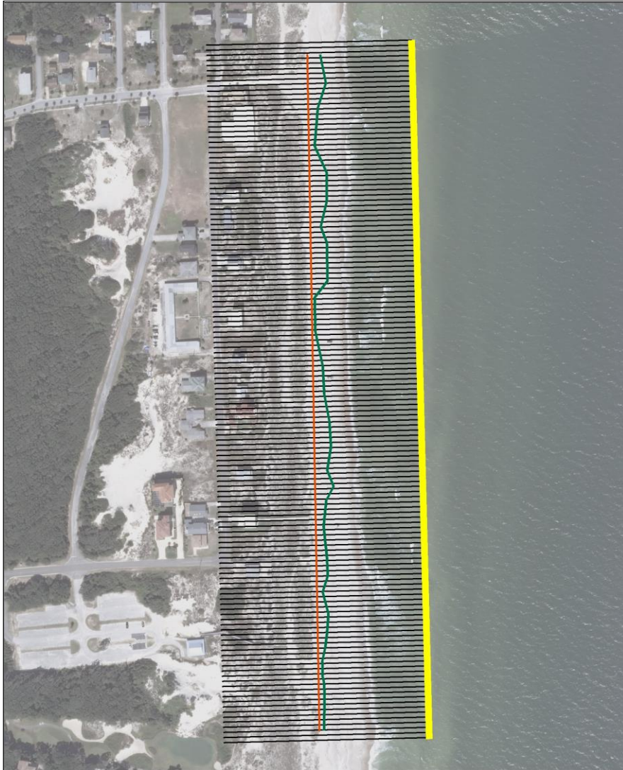
Figure 2. Example assessment at American Beach (TIMU) using mock shorelines. Neap-tide high-tide mock shorelines (orange and green) with DSAS analysis transects (black) and the baseline (yellow) are shown.
