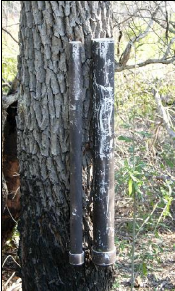
Figure 7. Pair of PVC pipes at Gulf Islands NS. One pipe in the pair is 2.5 cm [1-inch] in diameter and the other is 5 cm [2 inches] in diameter. All pipes are painted brown-grey for camouflage and to help standardize internal conditions, although paint may become slightly scratched and worn over time.
