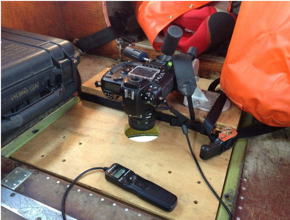
Figure SOP5.6. The above image illustrates the attachment of the digital camera to the tripod affixed to the custom platform that fits the belly port of the aircraft. The digital camera is aimed vertically, adjusted with a portable level in flight, and controlled with the attached remote timer.
