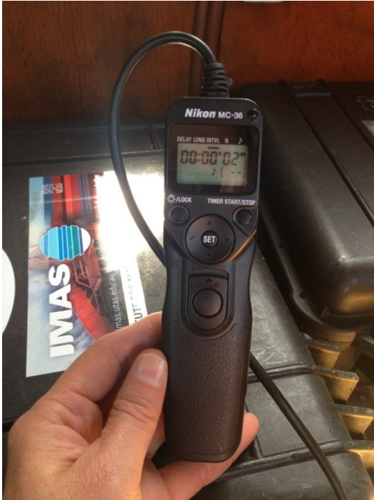
Figure SOP5.4. Nikon MC-36 remote timer programmed to trigger the digital camera once every two seconds.
