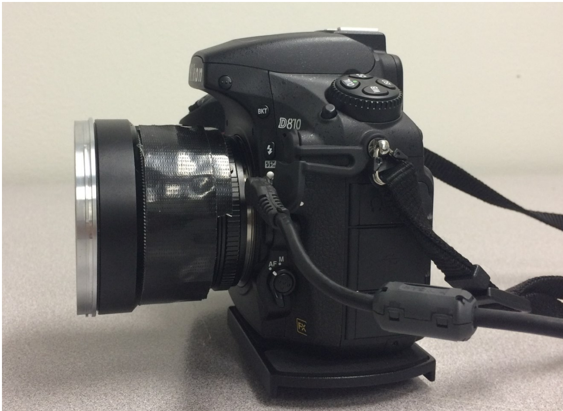
Figure SOP5.3. Nikon D810 digital camera with Zeiss 85mm lens attached. The lens focus is adjusted to infinity and taped in place. Also shown is the attachment port for the cord connecting the remote timer.
