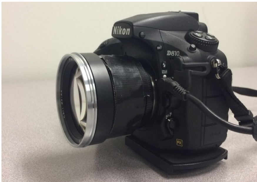
Figure SOP5.2. The above image shows the Nikon D810 digital camera with Zeiss 85mm lens attached and the focus taped to infinity. The attachment port for the cord connecting the remote timer is also shown.
