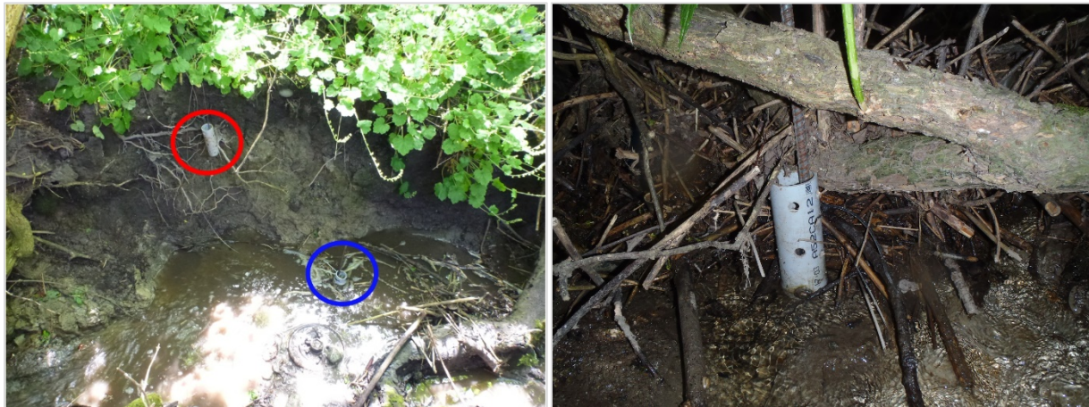
Figure 9. The position of the air (red circle) and water (blue circle) loggers as they were deployed in Ebey's Watercourse in 2013 (left), and the water logger as it was found during the 2014 site visit (right). Note: The gray cowlings holding the temperature loggers are 5 cm in diameter and 20 cm in length.
