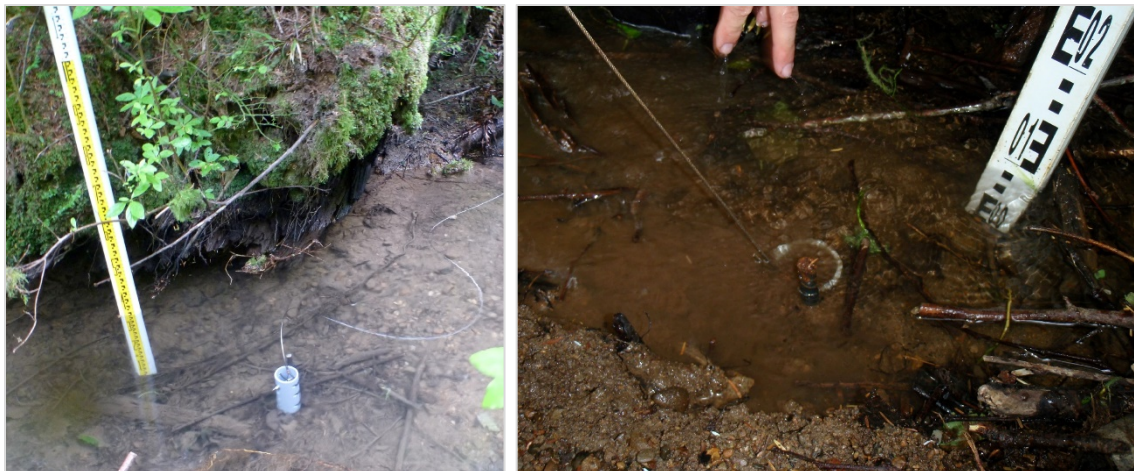
Figure 26. Photographs of the water logger installations in Megler Creek. The image on the left depicts the logger as installed in 2011, and the image on the right depicts the logger partially buried in sediment as found during the 2012 site visit.
