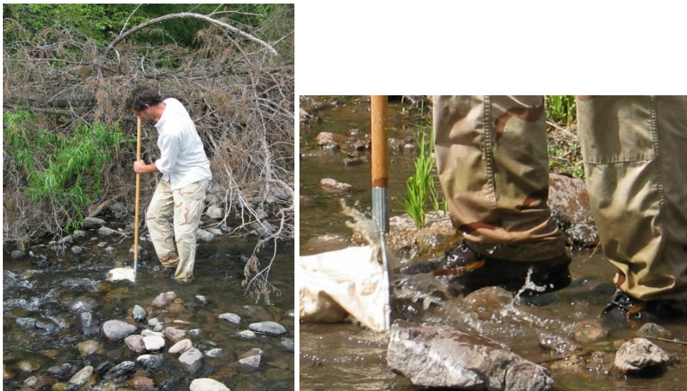
Figure 3. The kick net method involves dislodging macroinvertebrates upstream of the net by vigorously stomping in the channel substrate, the current areas them into the net.
