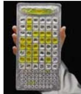
Figure 1. Photo instructions of the use of Quanti-tray®/2000 and Colisure® reagent
