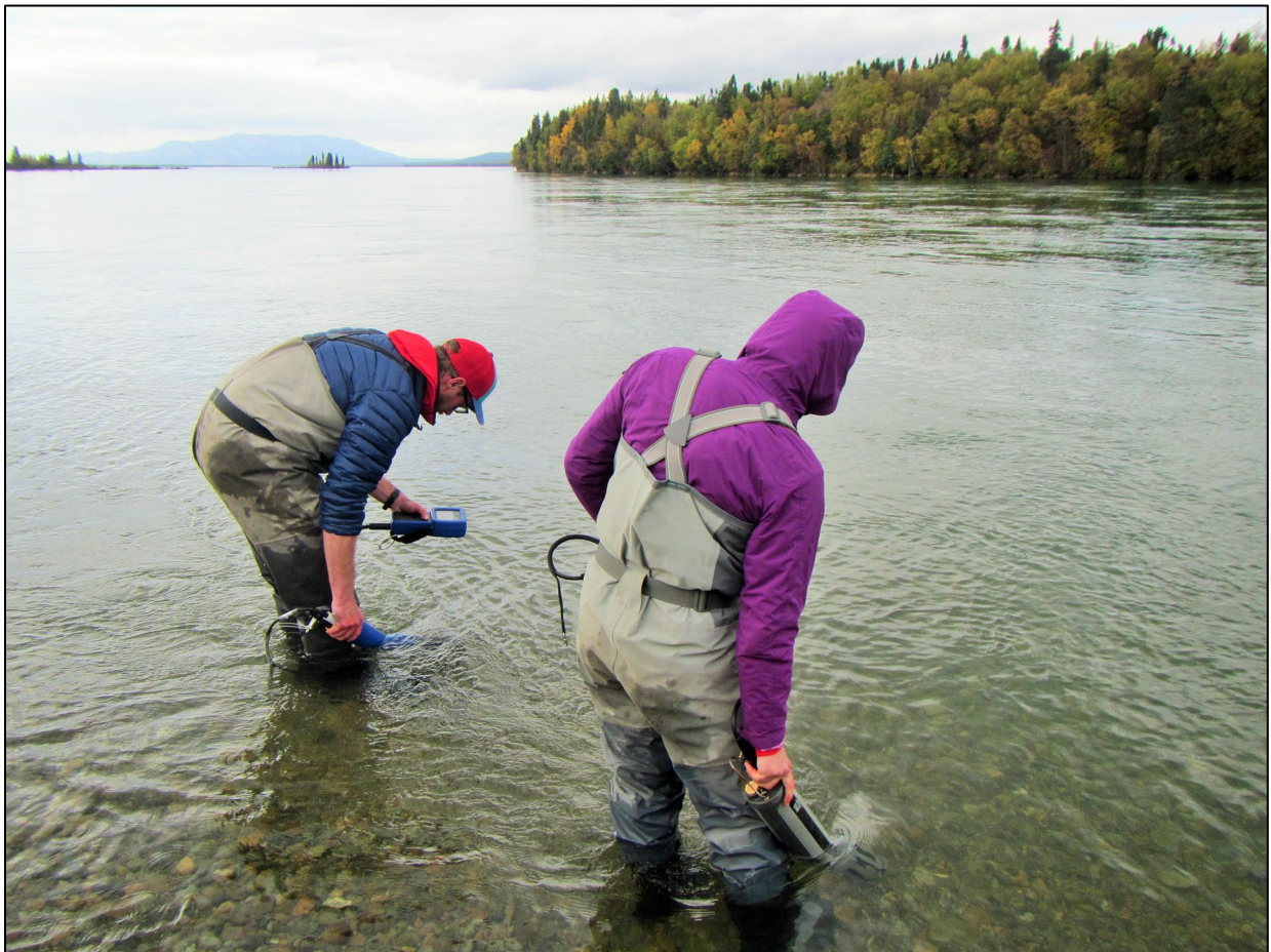
Figure 2. Evan Booher and Katie Junghans take side-by-side water quality measurements on September 15, 2016 to assess sensor fouling on the 6600 sonde deployed at the outlet of Lake Clark (NPS/KRISTA BARTZ).
