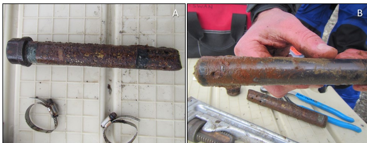
Figure 9. Biofouling and rust found on the housing (A) and level logger (B) at the outlet of Naknek Lake on May 2, 2016 (NPS/BOB PETERSON).
