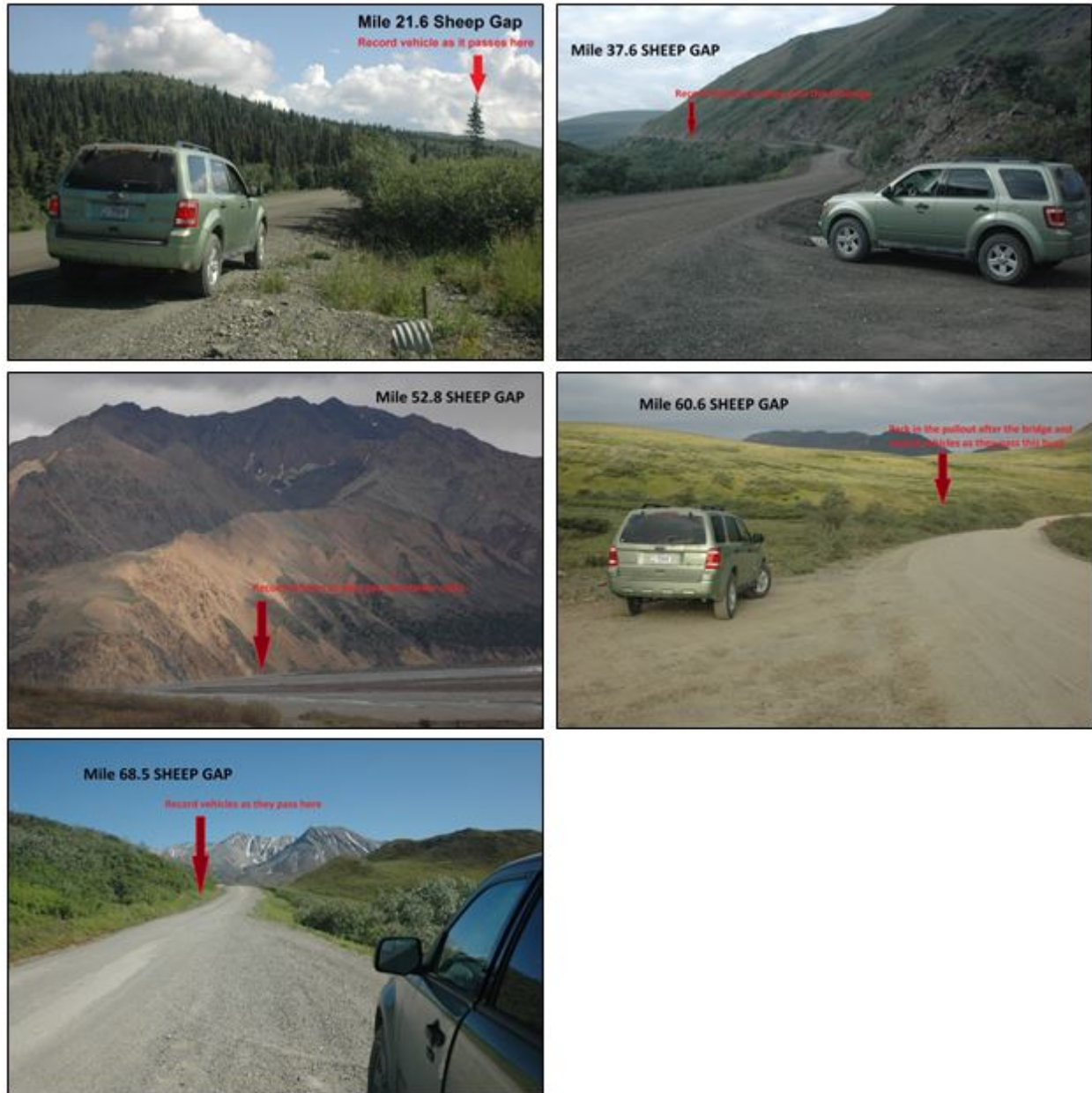
Figure 6. The spacing of traffic at five sheep crossing locations (i.e. sheep gaps) is used as an indicator to measure desired resource protection efforts along the Denali Park Road (Denali National Park and Preserve, Alaska, USA). Arrows indicate the monitoring reference point. The standard is a minimum percentage of hours that contain at least one 10-minute gap in traffic.
