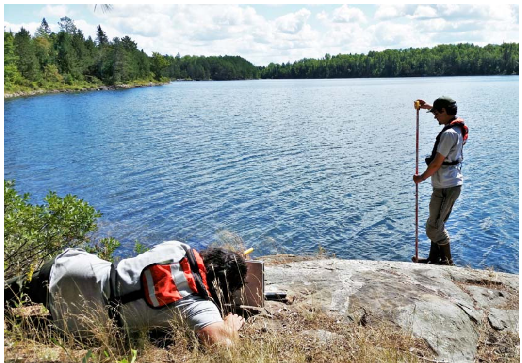
Biologists measure the water level on Cruiser Lake using a shoreline benchmark, an eye level, and a stadia rod. NPS PHOTO
