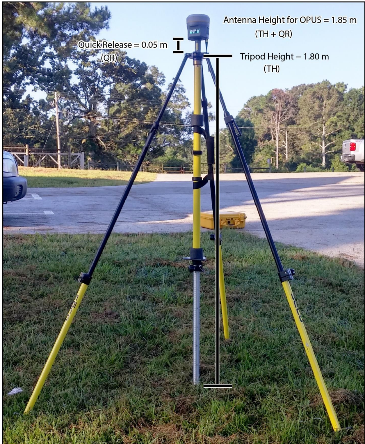
Figure 1. Antenna height that is specified when uploading to OPUS and OP should be the tripod height (TH) plus the 5 centimeter (2 inch) quick release (QR) if it was used.
