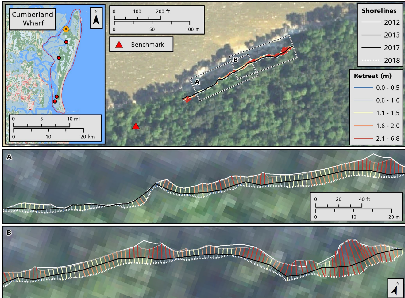
Figure 3. Island margin retreat at Cumberland Wharf.
