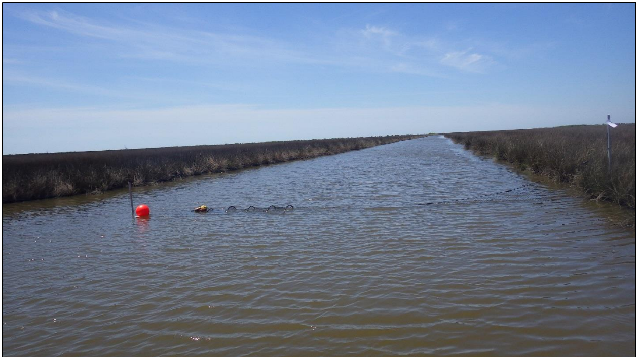
Fig. 6: Style 4 fyke net, a six hoop 1 \frac{1}{2} inch mesh coated net with a 25 foot lead, deployed in a Marsh Point inlet.
