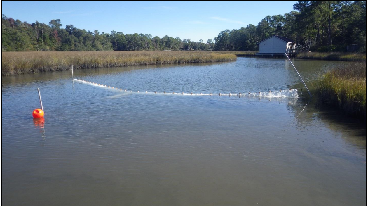
Fig. 3: Style 1 fyke net, a double wing, 1/8 inch nylon mesh with 2, 40 foot leads, and 4 hoops.
