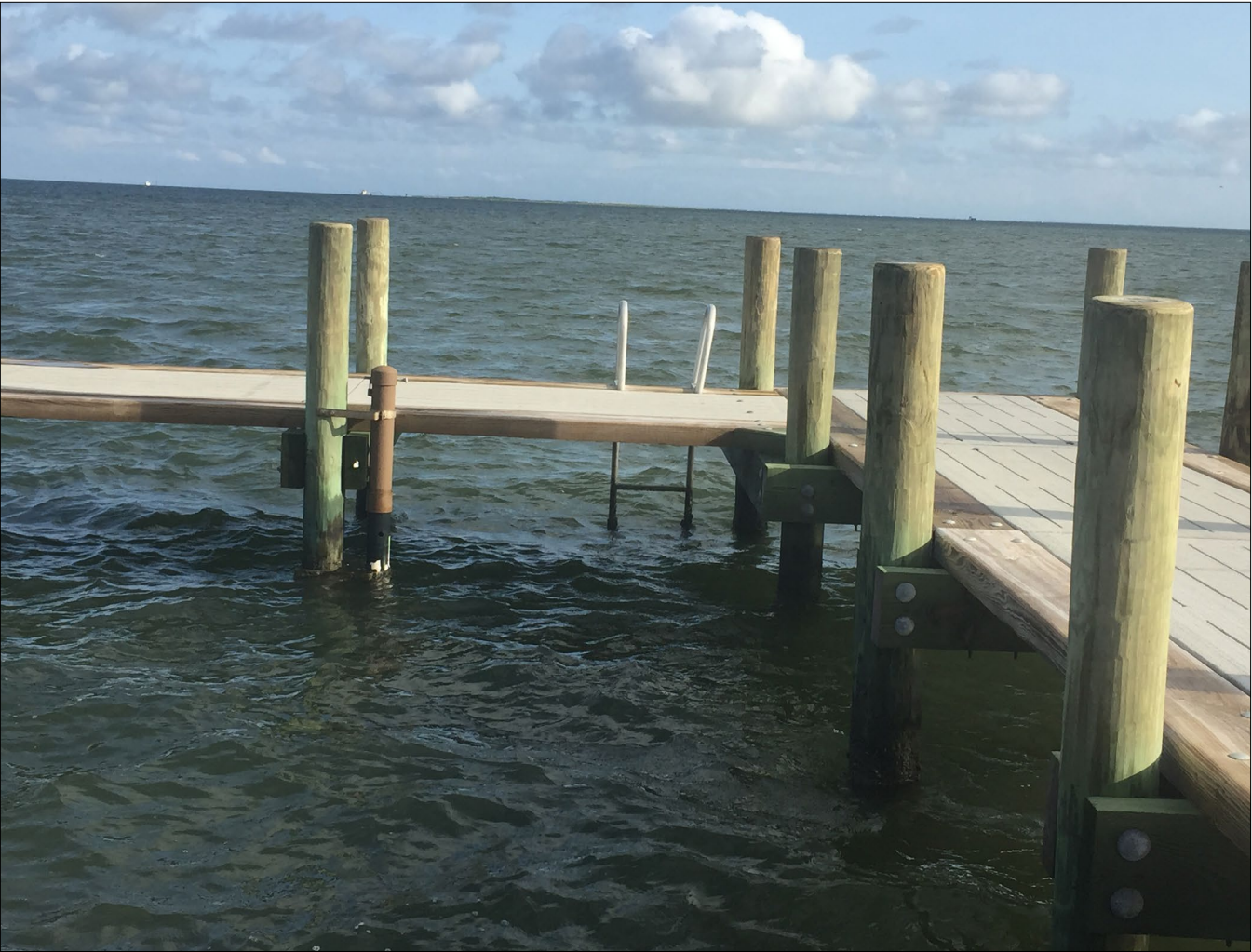
Figure 3. Continuous data collection platform on the Cape Hatteras National Seashore dock near the visitor center parking lot. NPS photo / Brian Gregory.
