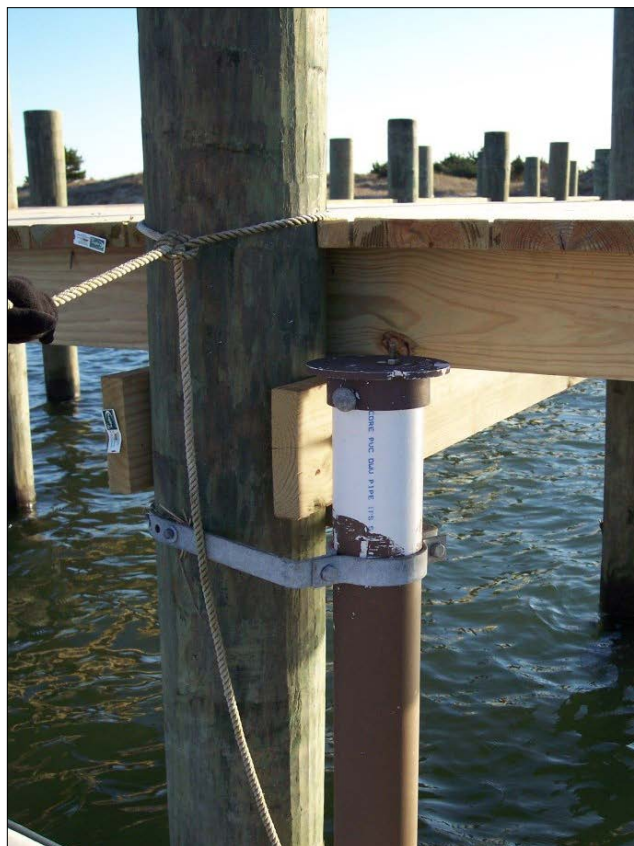
Figure 4. Photo of continuous data collection station at Shackleford Banks Dock (CALO01) at Cape Lookout National Seashore. NPS photo / John Fear.
