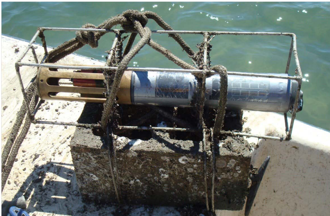
Figure 5. Photo of continuous data collection sonde and mount used at Middle Marshes (CALO2) at Cape Lookout National Seashore. NPS photo / John Fear.
