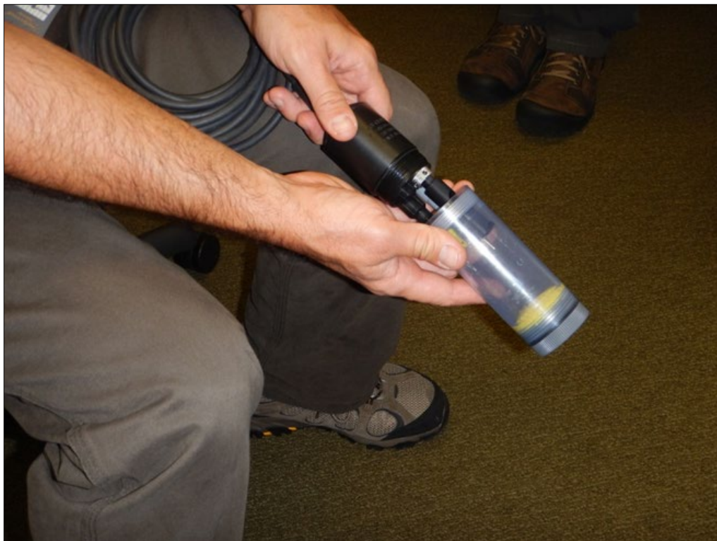
Figure SOP 5-3. After use, return the probe to the plastic storage cylinder with the yellow sponge (make sure the sponge is damp).
