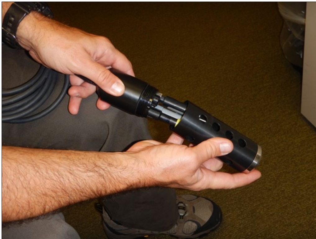
Figure SOP 5-2. Carefully thread the metal cylinder over the sensors before use.
