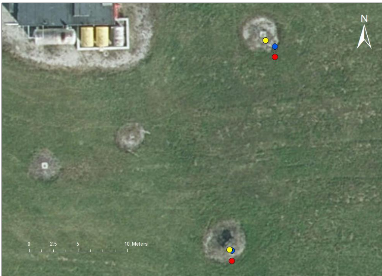
Figure SOP 13-3. Two test points taken with the Trimble GPS on the ground (yellow circles), hovering in a helicopter (red circles), and corrected for the antenna offset (blue circles).
