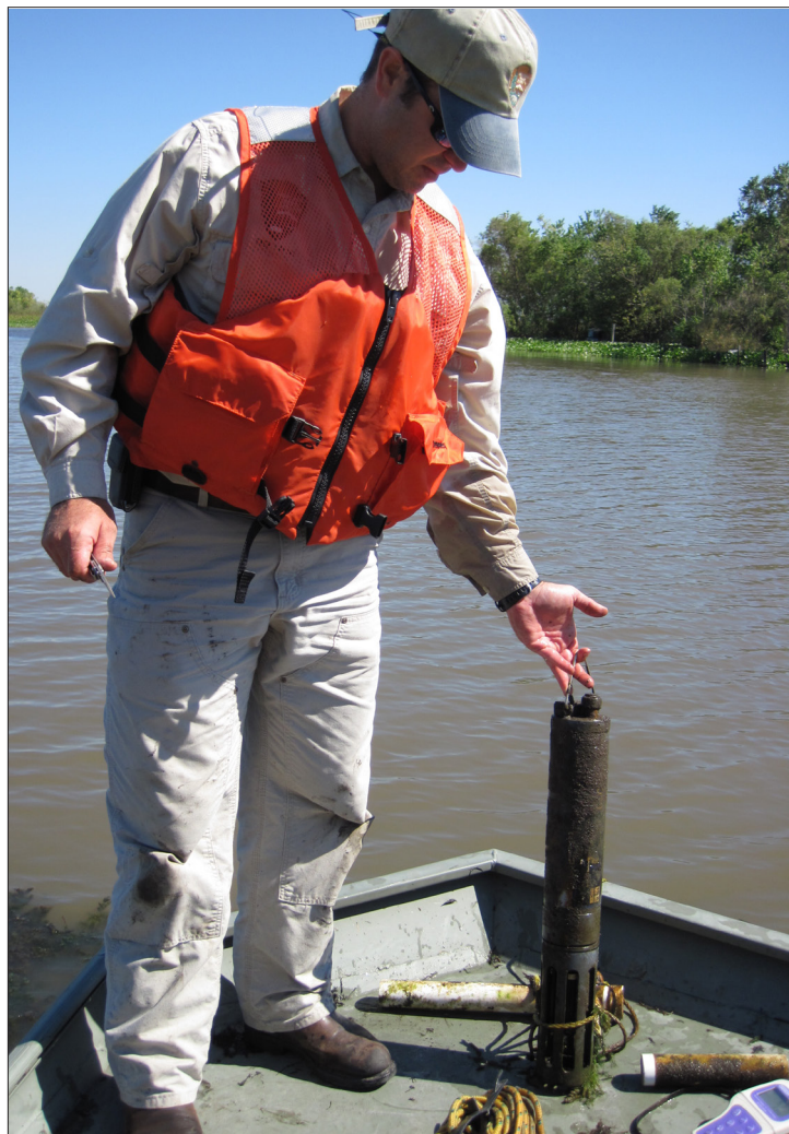
Above: A field crew member pulls a continuous data sonde from the water for maintenance.
