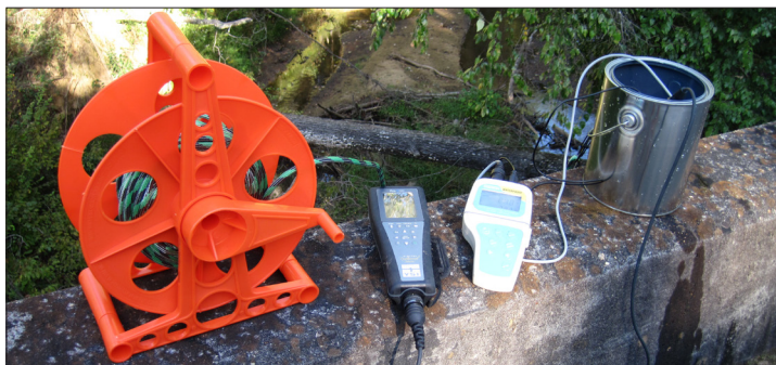
Tools for measuring water quality from a bridge where stream-side access is limited.
