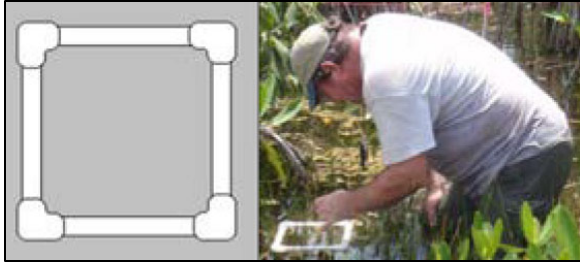
Figure B-7. Model of 20 × 20 centimeters (7.9 × 7.9 in) PVC frame placed on the ground centered inside of the desired quadrant.
