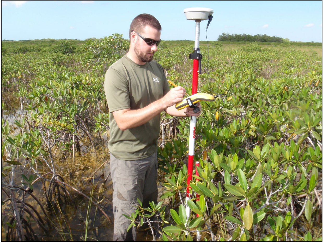
Figure B-3. Location of a point using the Trimble GeoXT.
