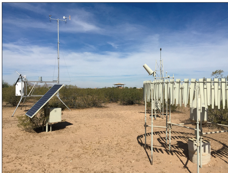
Figure 2-1. Weather stations at Casa Grande Ruins National Monument: A remote automated weather station, shown at left, and a high-precision regional climate reference network station, shown at right. A NOAA Cooperative Observer Program station is located near the Great House (seen in background).
