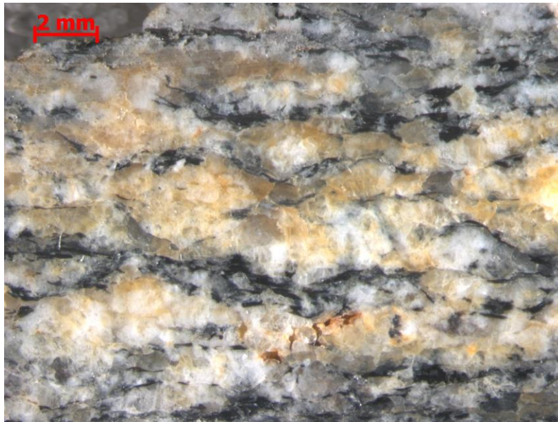
Figure 14. Magnified image of Stone Sample 2 showing the foliation highlighted by black biotite.
