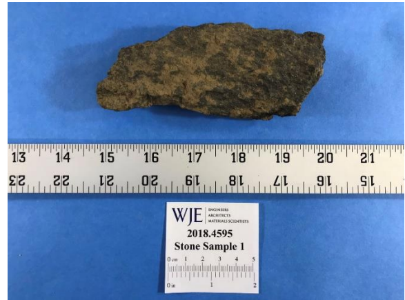
Figure 5. Images of Stone Sample 1, as-received. Note the overall dark brown to black appearance of the samples.
