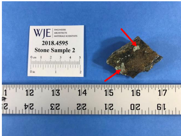
Figure 6. Images of Stone Sample 2, as-received. Note the overall dark brown to black appearance of the samples, as well as biological and/or organic growth (red arrows).
