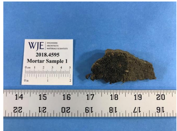
Figure 1. Images of Mortar Sample 1, as-received. Note the dark deposits on the surface of the mortar in the right image.
