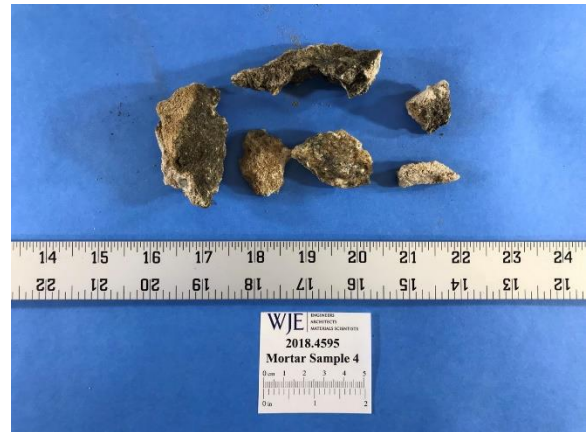
Figure 4. Images of Mortar Sample 4, as-received. Note the dark deposits on the surfaces of the mortar in the images.
