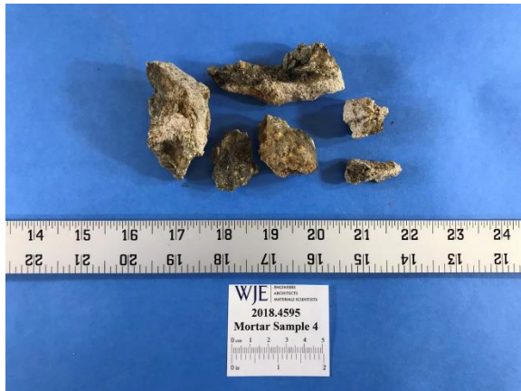
Figure 4. Images of Mortar Sample 4, as-received. Note the dark deposits on the surfaces of the mortar in the images.
