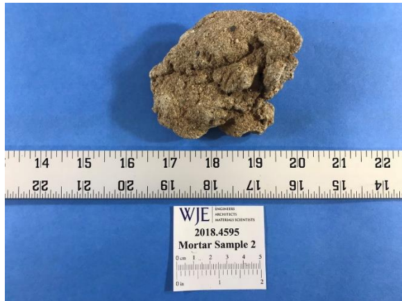
Figure 2. Images of Mortar Sample 2, as-received. Note the dirt deposits on the surface of the mortar in both images and the beige coloration of the samples.
