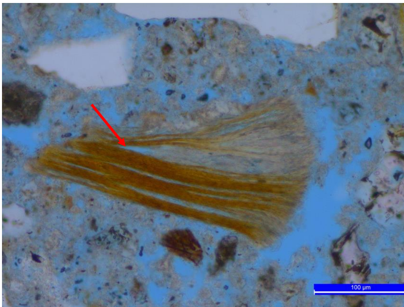
Figure 12. Mortar Sample 2 exhibits a porous paste structure, as shown by the absorption of a large amount of blue dyed epoxy (the overall blue coloration of the image). Red arrow points to biotite mica, part of the sand within the mortar.
