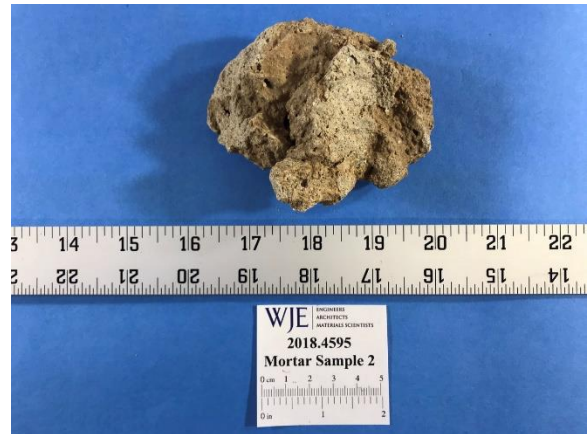
Figure 2. Images of Mortar Sample 2, as-received. Note the dirt deposits on the surface of the mortar in both images and the beige coloration of the samples.
