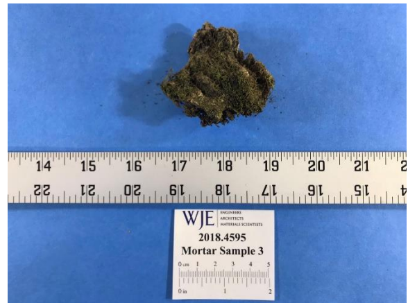
Figure 3. Images of Mortar Sample 3, as-received. Note the dark deposits on the surface of the mortar in the images.
