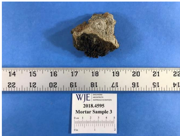
Figure 3. Images of Mortar Sample 3, as-received. Note the dark deposits on the surface of the mortar in the images.
