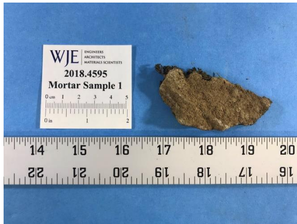
Figure 1. Images of Mortar Sample 1, as-received. Note the dark deposits on the surface of the mortar in the right image.
