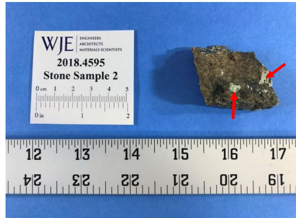
Figure 6. Images of Stone Sample 2, as-received. Note the overall dark brown to black appearance of the samples, as well as biological and/or organic growth (red arrows).
