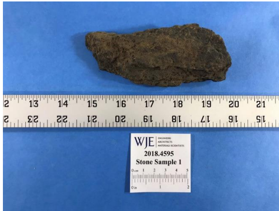
Figure 5. Images of Stone Sample 1, as-received. Note the overall dark brown to black appearance of the samples.
