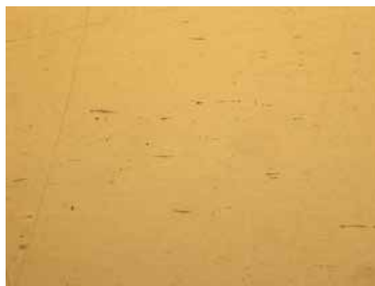
Figure 3: Micrograph of manganese sulfide stringers in the plate, W1, as-polished condition. (256x) (Photo taken by TMR in 2014)
