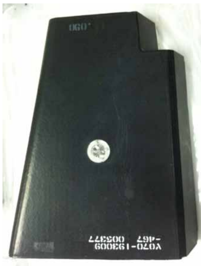
Figure 10: Space shuttle HRSI tile. (Credit: Joseph Sembrat, Conservation Solutions, Inc., 2004)
