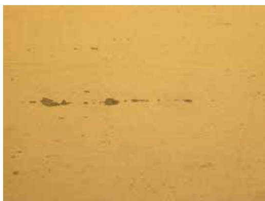
Figure 2: Micrograph of a plate inclusion, W1, as-polished condition (517x) (Photo taken by TMR in 2014)
