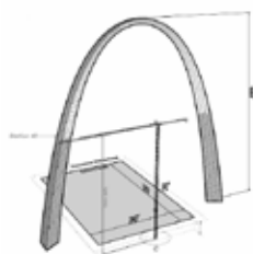
Figure 21: The access survey revealed that the highest access from the ground would be 344 feet using a guyed crane tower and boom lift.
