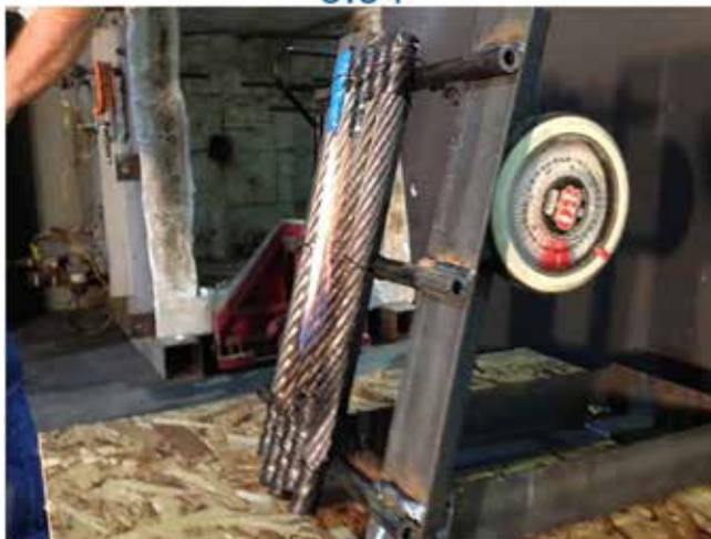
Figure 5. Ignition and self-extinguishment of cable
