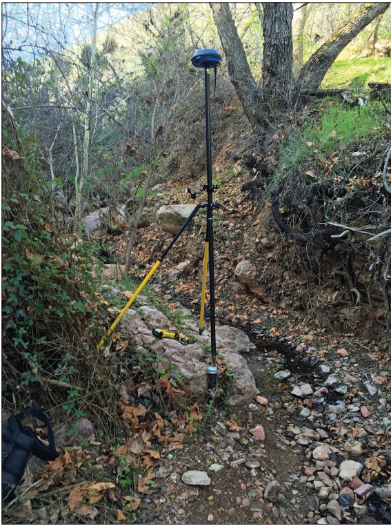
Figure 3-2. Piezometer at the shallow groundwater monitoring site, Cave Canyon Creek, Tonto National Monument. NPS/Jacob DeGayner.
