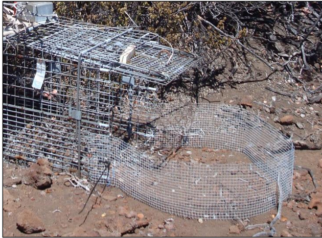
Figure 19. Cage trap outfitted with a “goose guard.”
