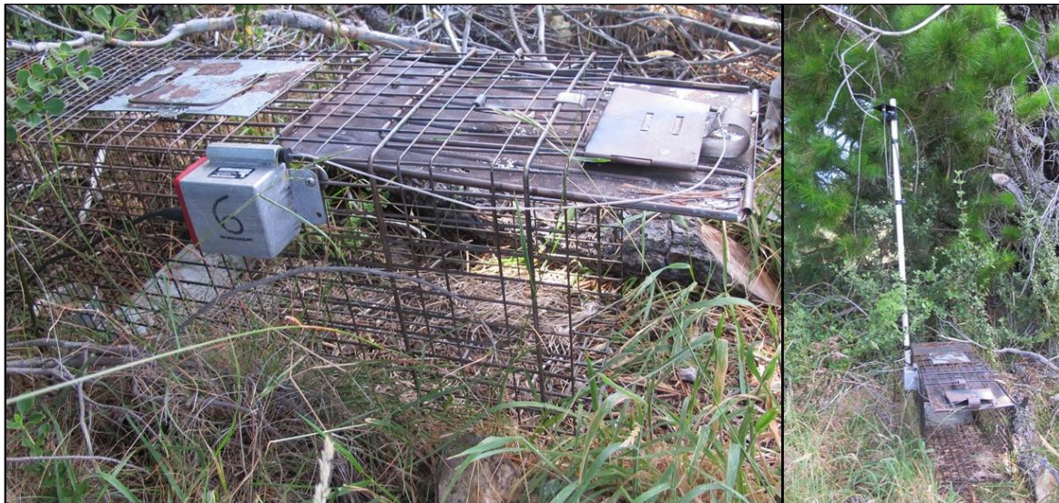
Figure 20. Cage trap with VHF telemetry Trap Monitoring System (TMS).
