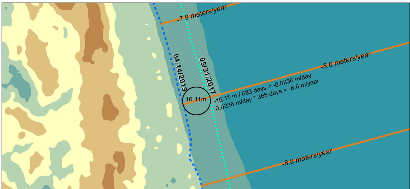
Figure 2. End Point Rate calculation for transect at Padre Island NS. In this case the shoreline retreated 16.11 meters (52.85 ft) over 683 days, or 8.6 meters (28.2 ft) of retreat per year.
