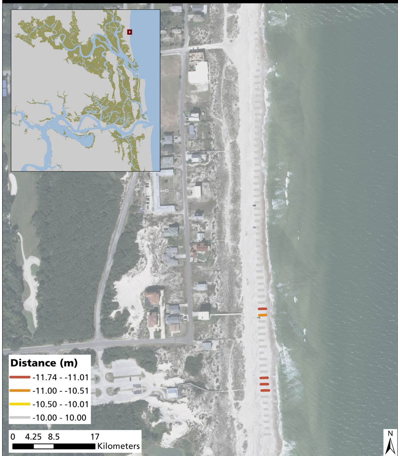
Figure 3. Map of shoreline change distance (meters) for the 2018 and 2019 surveys collected at American Beach at Timucuan EHP&P. The more negative shoreline change denotes more erosion and is shown in warmer colors. The less negative shoreline change denote less erosion and in some cases can represent accretion (when positive) and is displayed as cooler colors. The grey transects denote shoreline change distance within the uncertainty range of the data ( \pm 10 meters).
