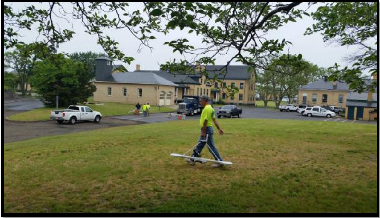
Figure 5.2: Paul McLeod carrying out the EM survey at the Sandy Hook lighthouse. The photo is looking southwest away from the lighthouse.
