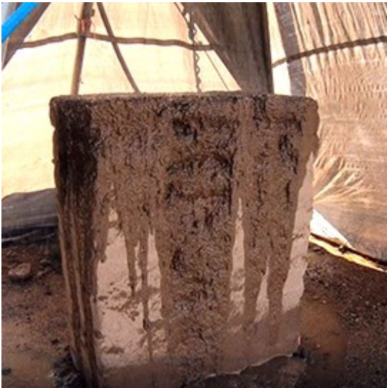
Walls were subjected to simulated rainstorms of different intensity based on the historical climate record.
