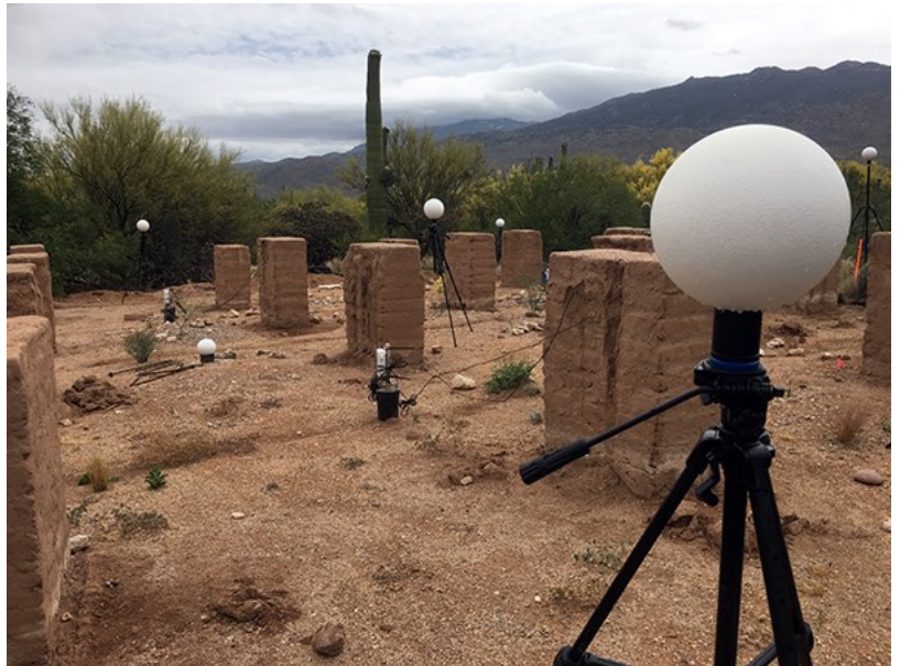
White globes served as reference points to maximize accuracy during LiDAR scanning.
