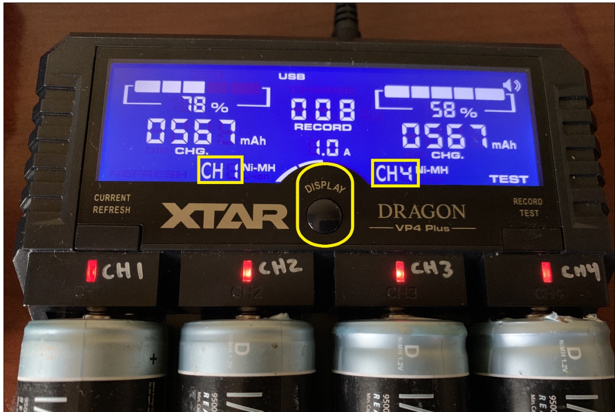
Figure 3. XTAR Dragon VP4+ battery charger display screen. Display button (center) and channel indicators (left and right) are indicated by yellow boxes.
