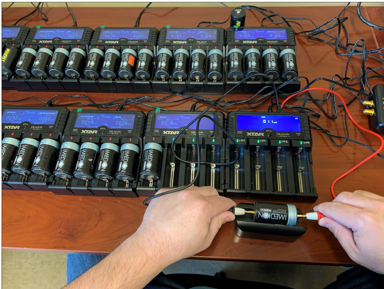
Figure 4. A business card holder makes an excellent battery testing cradle in which to support the battery as the test leads are applied for voltage and internal resistance testing.
