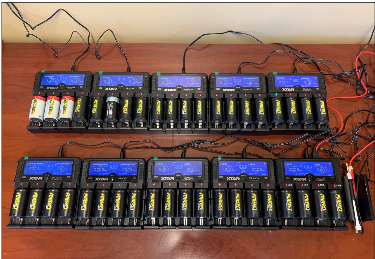
Figure 5. A group of 40 D-cell batteries are mounted in ten XTAR Dragon VP4+ chargers to undergo capacity testing. A pair of test leads is placed in a testing cradle to the lower right.
