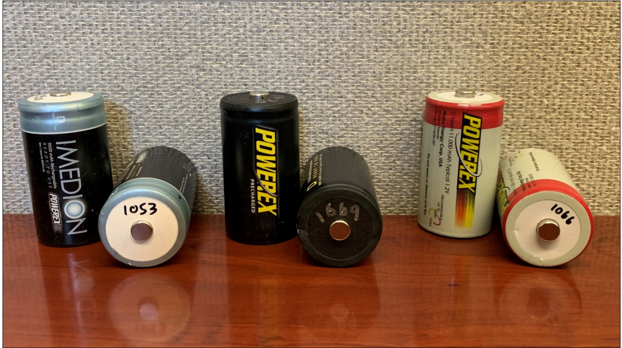
Figure 1. Three types of D-Cell NiMH batteries are currently used with ARDs: (left) Imedion by Powerex, 9,500 mAh at 1.2 V; (center) Powerex black-top, 10,000 mAh at 1.2V; (right) Powerex red-top, 11,000 mAh at 1.2V. The Imedion and Powerex red-top batteries have been discontinued by the manufacturer and are being phased out of project usage.
