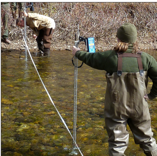
Scientists taking a cross-section streamflow measurement for the Devils Postpile Gage. Photo by: Alice Chung-MacCoubrey.
