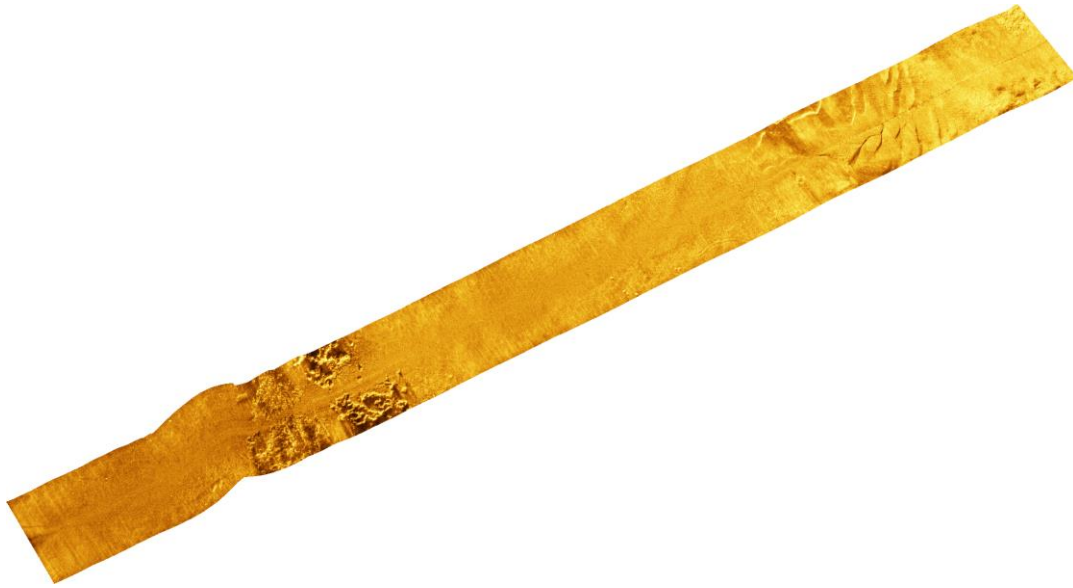
Figure 7. An example of an individual track line image displaying processed sidescan data (i.e. central nadir region removed and color balanced). The sidescan data shown are from the Fire Island National Seashore benthic habitat mapping project.
