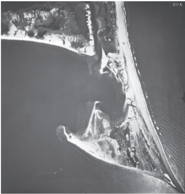
Figure 5. View of Cape Lookout Bight in 1941, showing the dramatic changes precipitated by construction of the breakwater just before World War II. (CALO Collection)
