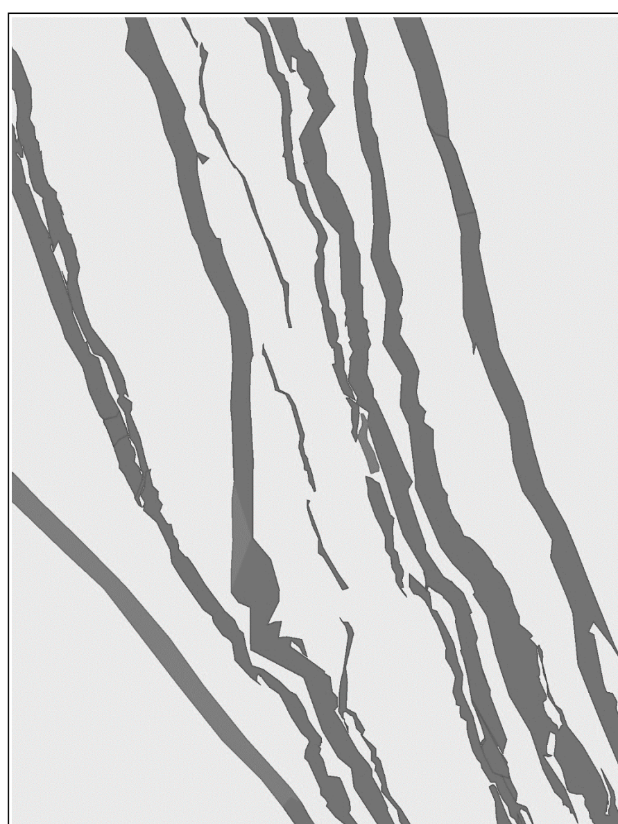
Details of a dike swarm NW of Schoodic Point created using survey techniques with RTK GPS rovers and tripod-mounted electronic total stations.
