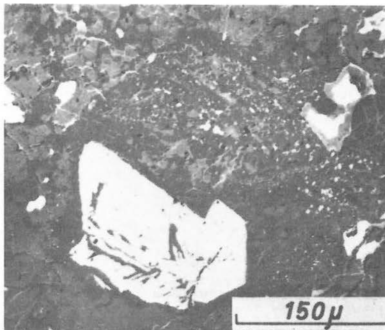
FIG. 20. Skeletal crystal of chromite in chondrule from equilibrated Cavour meteorite, as seen in reflected light. The photo is reprinted from Ramdohr (1973) with permission (see Acknowledgements).
