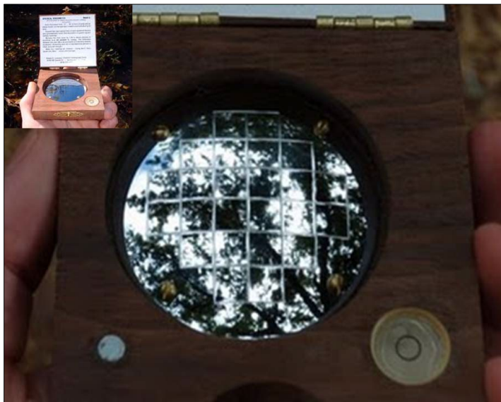
Figure 1. A spherical densiometer grid, illustrating how users visualize a dot in each corner of the grid (n=96 dots) and count the number of dots covered by canopy. Note the directions printed on the lid in inset photo.
