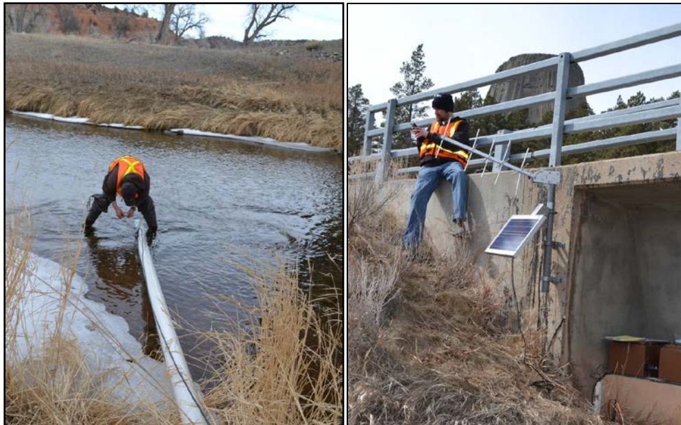
Figure 3. A researcher deploys a sonde device in 2013 to measure water quality on the Belle Fourche River at Devils Tower, WY (right panel). The United States Geological Survey Belle Fourche River gaging station (06427850) is set up for real-time data transmission via satellite. Photographs courtesy of NPS.
